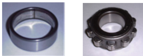
(a) Outer race flaw (b) Roller race flaw
