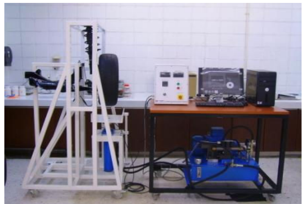
Fig. 6. Durability test rig for laboratory data measurement.
