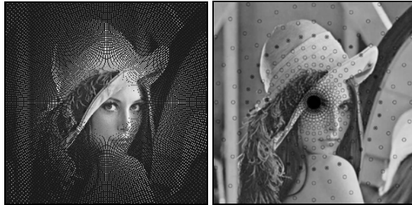
a. Points retained by EPT; b. Points retained by LPT Fig.2. Experimental images which indicate the points, retained after EPT and LPT
