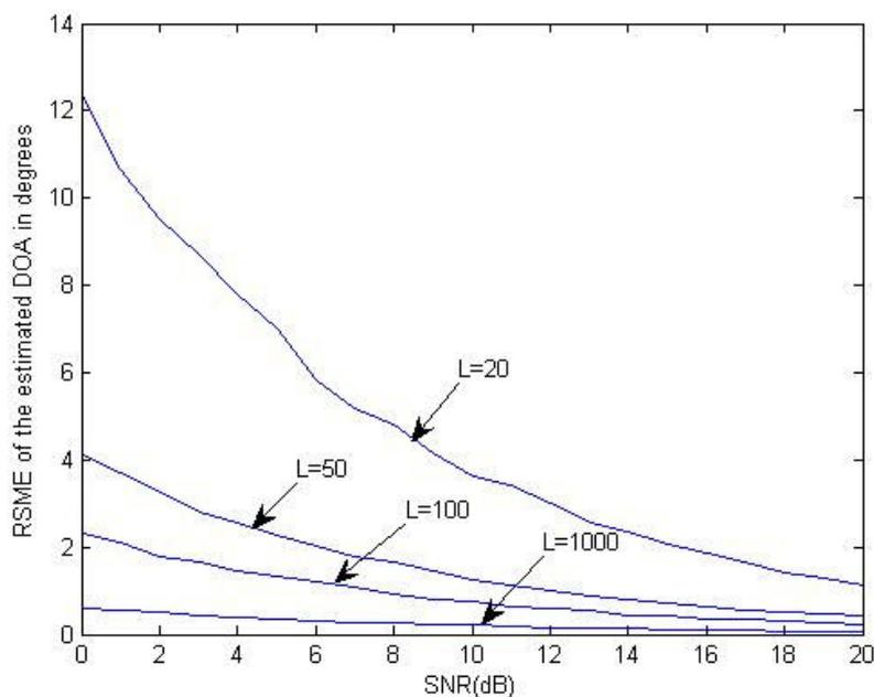
Fig.8. Root mean square error of the estimated DOA for different snapshot length  $L$  and the SNR of signal  $360^\circ$  of coverage in azimuth plane. And computer
