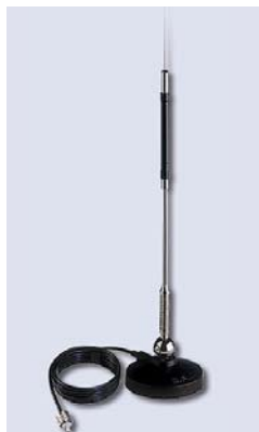
Fig. 6: Used \lambda/4 monopole receive antenna
