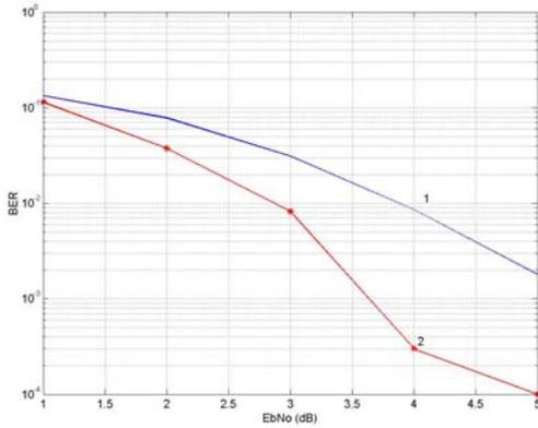
Fig.2 A comparison of performances of the SDFE and SOVA based turbo equalizer for a channel with fast exponential decay.
