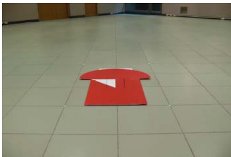
Fig. 12 Photograph of area measurement, the condition is as follows Shooting angle=45°
