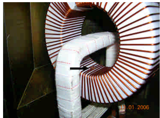
Fig. 3 VL on the low-voltage side of CRCT
