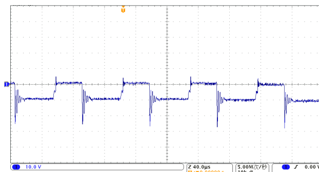
Fig.1 Terminal voltage waveform of DC motor
