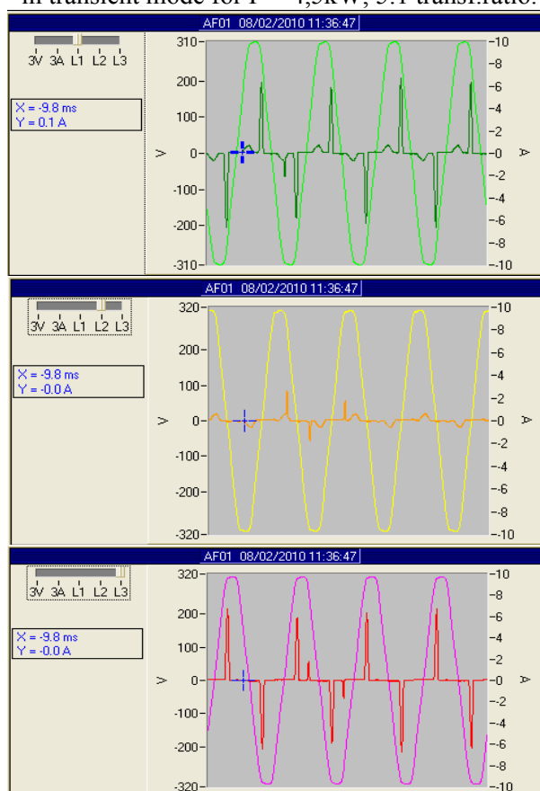
Fig. 3. Variation of the phase voltage and currents in transient mode for P = 9kW , 5:1 transf.ratio.
