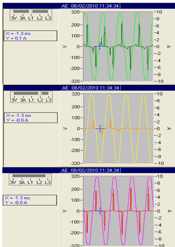
Fig. 2. Variation of the phase voltage and currents in transient mode for P = 4,5kW , 5:1 transf.ratio.
