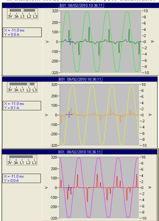
Fig. 5. Variation of the phase voltage and currents in transient mode for P = 4,5\text{kW} , 3:1 transf.ratio.
