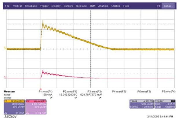
Fig. 22 Lightning Surge waveform used in experiments.
