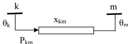
Fig.1. Transmission Line DC Power Flow Model
