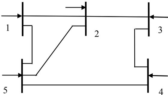
Fig.3. 5-Bus 6-branch sample System
