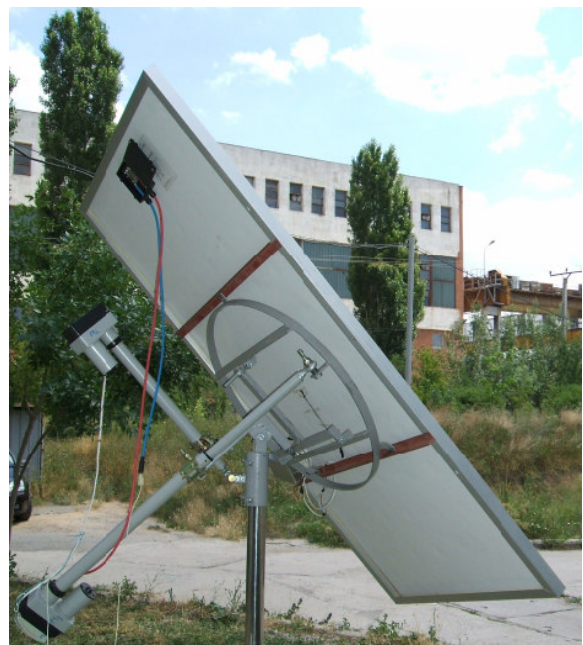
Fig.7 "Pseudo-equatorial" system for PV panel orientation
