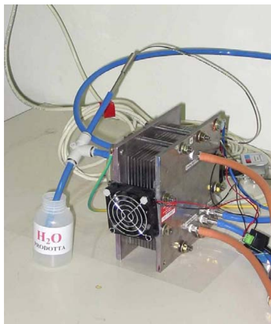
Fig. 2 One of the PEM FC stack under test
