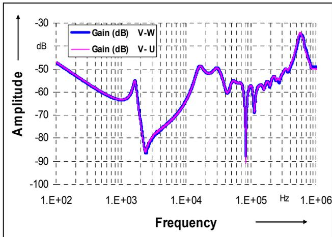
Fig.10: FRA measurements between the high voltage windings for normal transformer
