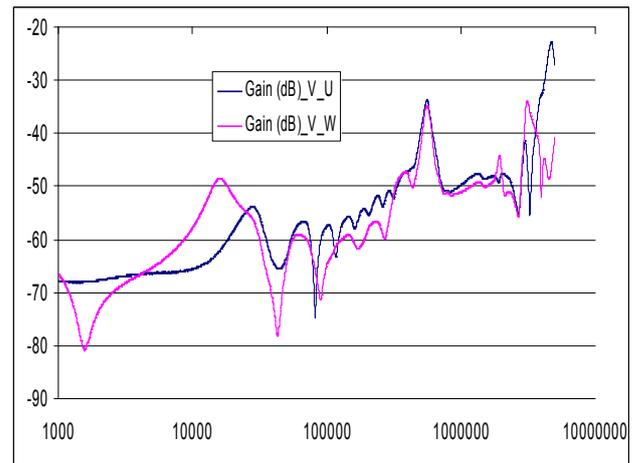
Fig. 8: FRA measurements between the high voltage windings for faulty transformer.
