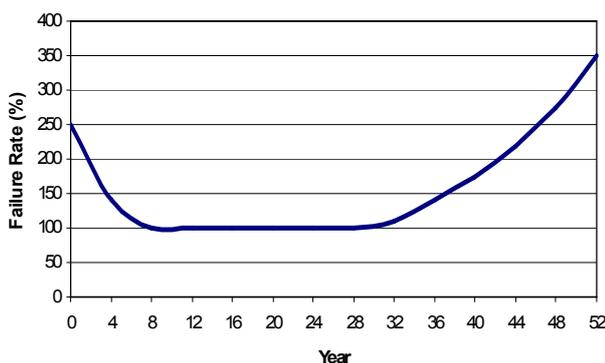
Figure 1 – Bath-tub Failure Curve for Power Transformers [2]
