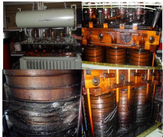
Fig. 12: A picture group of the transformer opening process.
