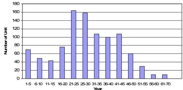
Figure 2 – Age Distribution Profile for Power Transformer [2]
