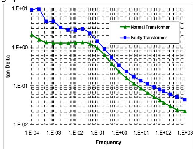
Fig. 6: PDC measurements for the faulty and normal transformer
