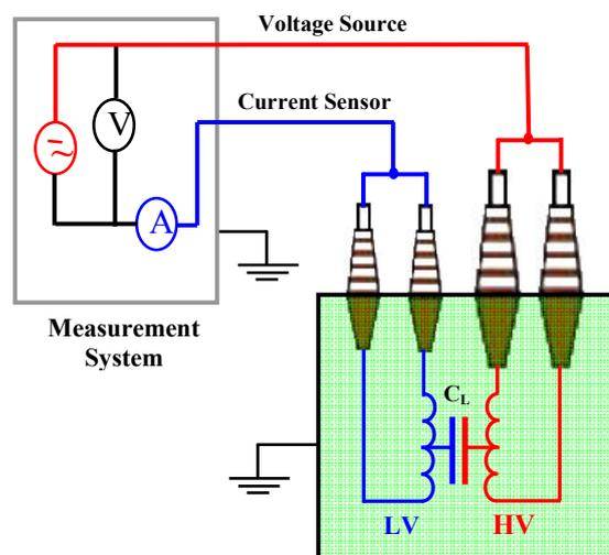
Fig.5: Schematic diagram of the PDC measurements connections.
