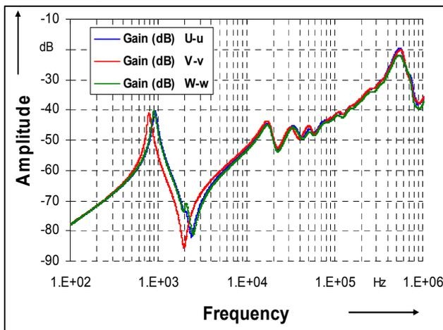
Fig.11: FRA measurements between the high – low voltage windings for normal transformer
