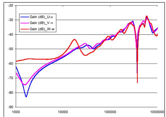
Fig. 9: FRA measurements between the high – low voltage windings for faulty transformer.
