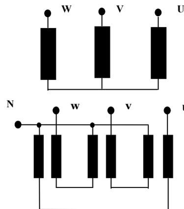
Fig. 4: Transformer schematic diagram, (YZ-5).
