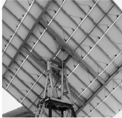
Fig. 3. Dual axis polar mounted solar tracker
