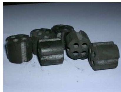
Fig. 9 The pieces of nickel catalysts after experiments
