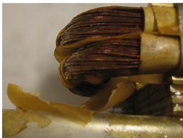
Fig. 2. Motorette number 5 after the exposure to water at 150 °C. Note that impregnation is still very thorough.
