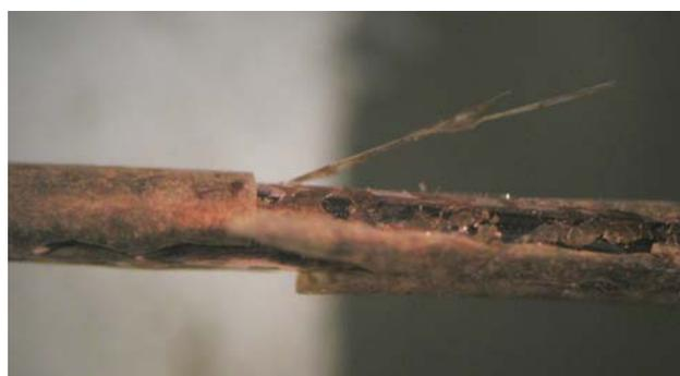
Fig. 5. Polyester-imide- and polyamide-imide-insulated wire after the exposure to hot, pressurized water. There is only a slight attachment between the insulation and the copper conductor. From most parts, the insulation has already decomposed.
