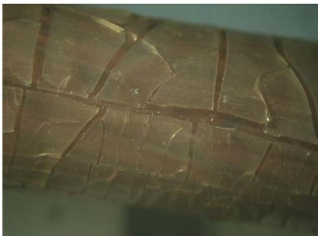
Fig. 6. PVC-insulated wire after the hot, pressurized water exposure. The surface of the insulation has suffered from severe cracking.
