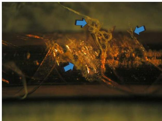
Fig. 4. Kapton polyimide-insulated wire from the point of a cut made in advance. Oddly-shaped strings marked with arrows are Kapton that has come off from the wire.
