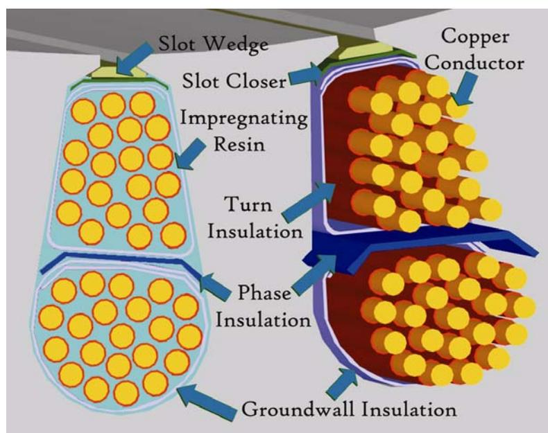
Fig. 1. Structure of the stator insulation system in the stator of a low-voltage, random-wound machine.
