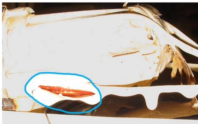
Fig. 3. Motorette number 2 after the tests. Note a huge crack.
