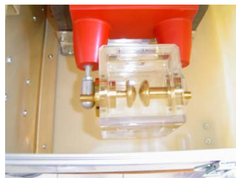
Fig. 2 Electrode for measuring the breakdown voltage of liquid insulation
