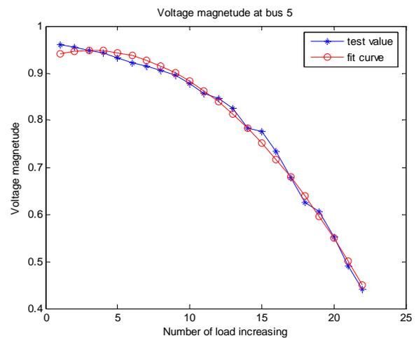
Fig. 10 Voltage magnitude of bus 5 versus time counter
