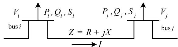
Fig. 3 Simple two-bus power system for LQP
