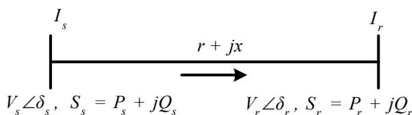
Fig. 2 Simple two-bus power system for  $L_{mn}$
