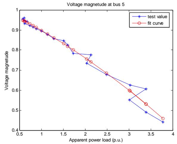
Fig. 9 Voltage magnitude of bus 5 versus load power
