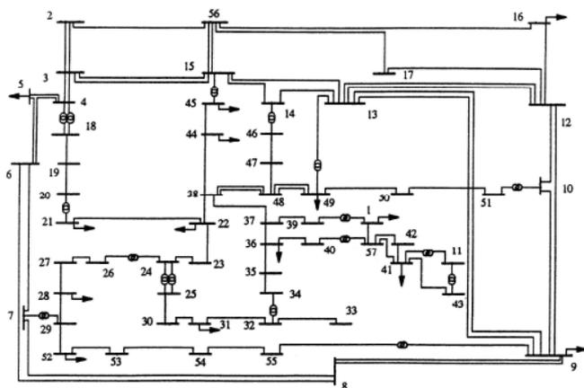
Fig. 21 Standard IEEE 57-bus test system
