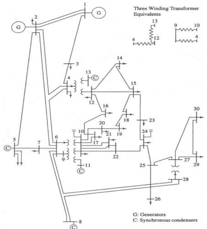
Fig. 14 Standard IEEE 30-bus test system
