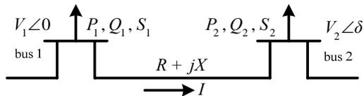
Fig. 1 Simple two-bus power system for FVSI
