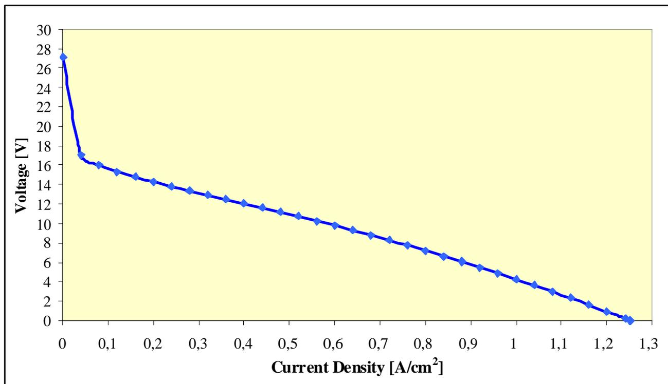
Fig.5 Polarization curve in the whole range of values
