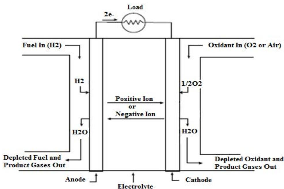
**Fig. 1 Operation of a PEM fuel cell**
