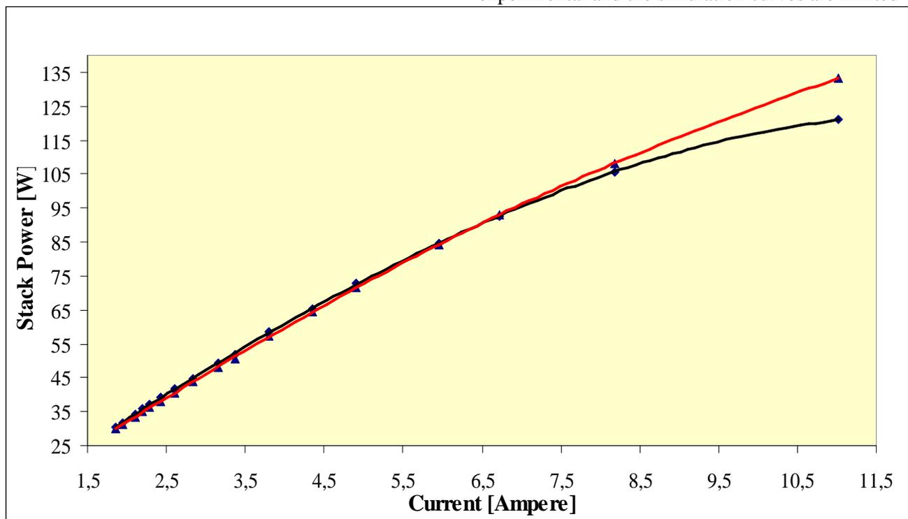
Fig.4 Experimental and theoretical Stack Power curve
