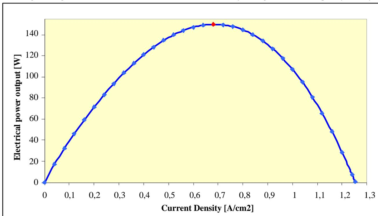
Fig.6 Stack Power curve in the whole range of values
