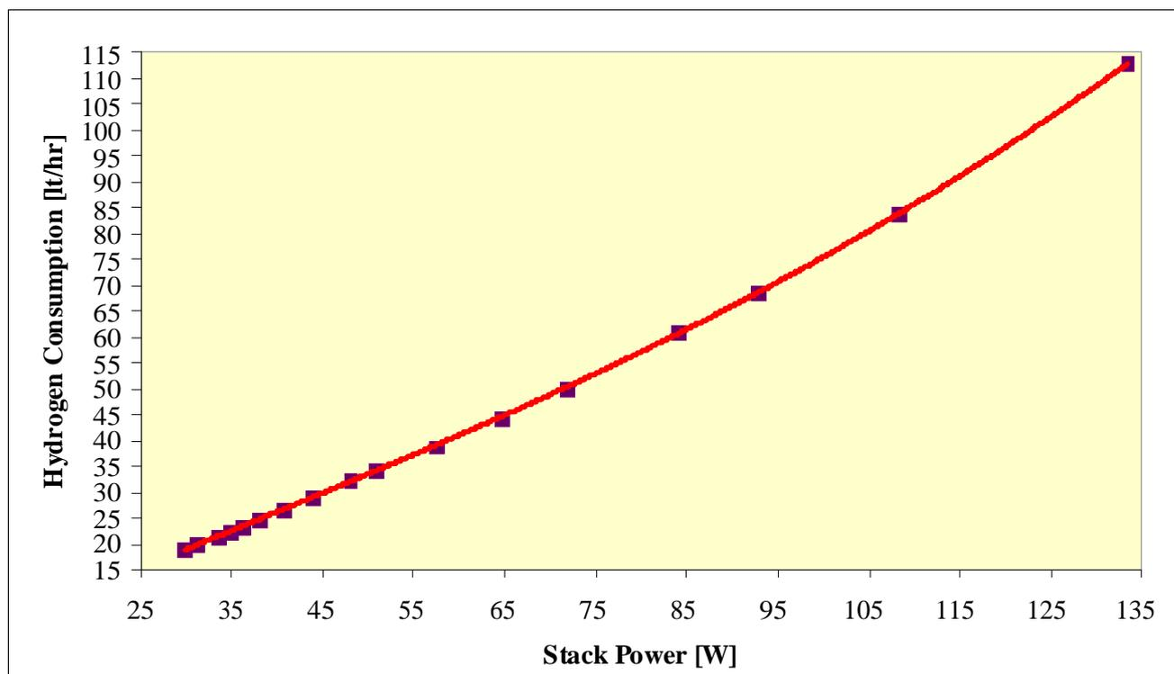
Fig.8 Hydrogen consumption as a function of Stack Power Output
