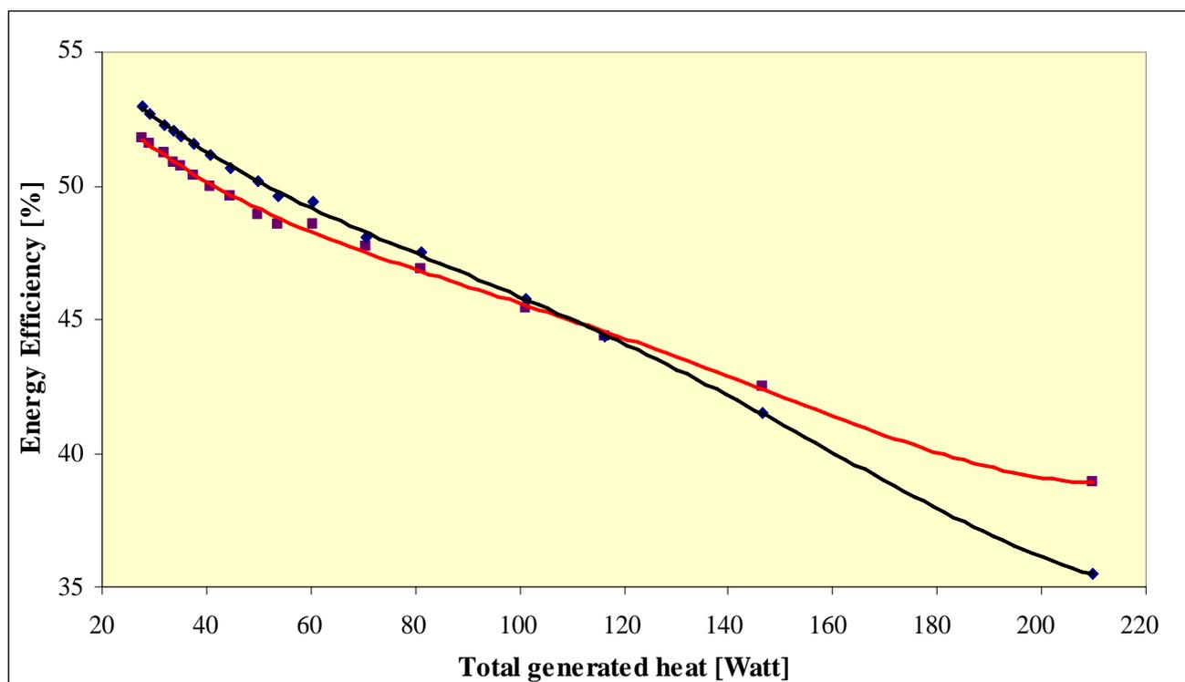
Fig.7 Energy Efficiency as a function of Total generated heat
