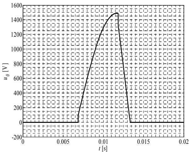
Fig. 9. Voltage between the star centers during the three-pole interruption of the network in Fig. 6.
