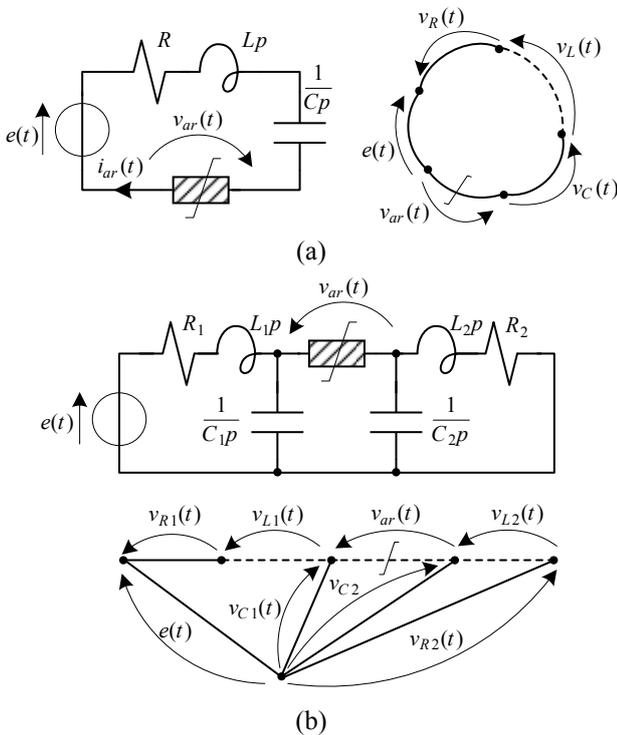
Fig. 2. Interrupted single-phase network. Case in which the electric arc must be put on the tree (a) and on the co-tree (b).
