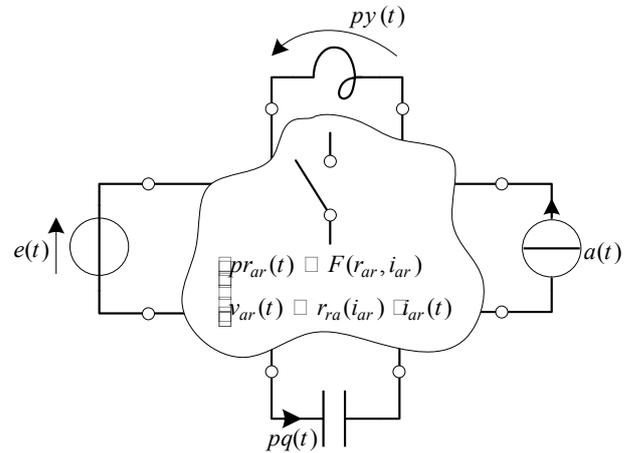
Fig. 1. The systemic interpretation of a single-phase network in which an electric arc is present.
