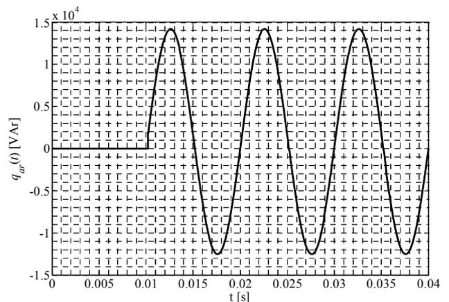
Fig. 11. Imaginary power obtained for the single-phase interruption process of the network in Fig. 6.
