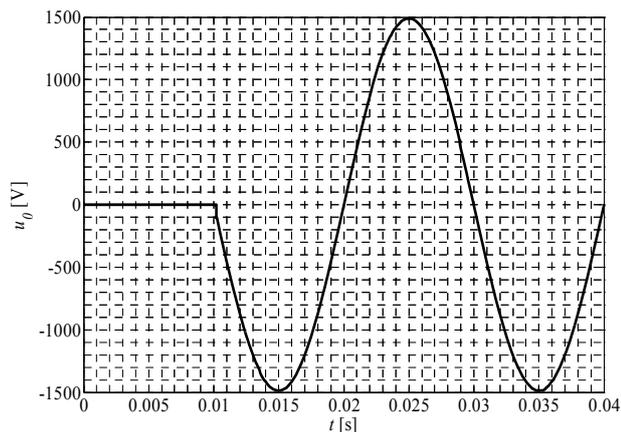
Fig. 12. Voltage between the star centers for the single-phase interruption of the network in Fig. 6.
