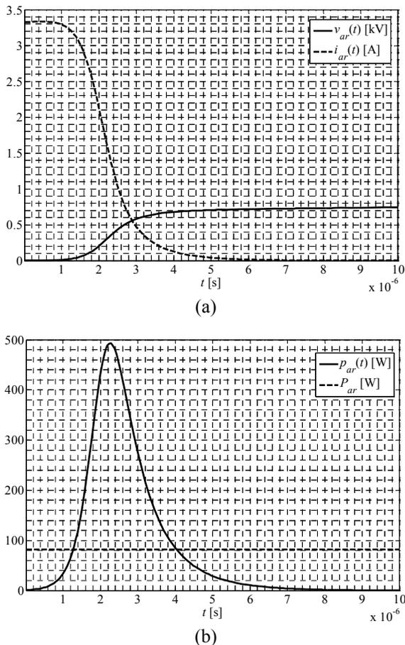
Fig. 4. (a) Arc voltage and current and (b) instantaneous power for the breaker in the single-phase network of Fig. 2.
