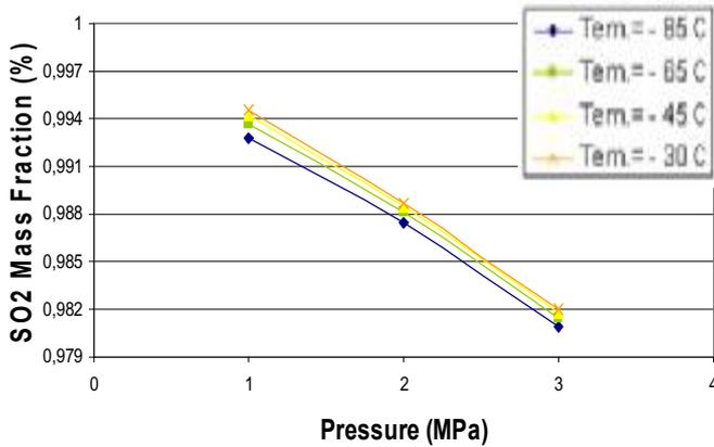
Fig. 6 Comparison of  $SO_2$  mass fraction at different conditions at the outlet of  $SO_2/O_2$  separation system
