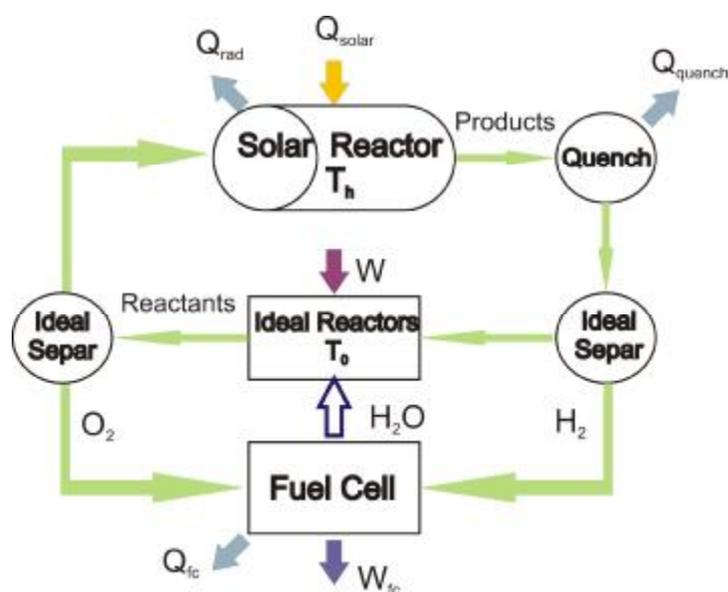
Fig. 1 Schematic model of solar energy conversion
