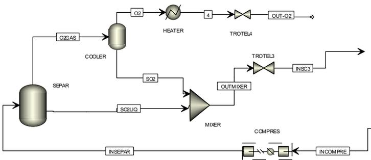
Fig. 3 SO<sub>2</sub>/O<sub>2</sub> separation – optimized sub-system of the WH cycle
