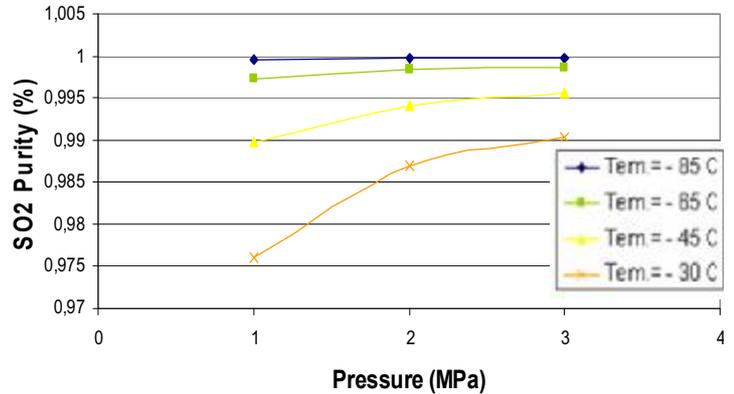
Fig. 4 Comparison of SO<sub>2</sub> purity at different conditions at the outlet of SO<sub>2</sub>/O<sub>2</sub> separation system
