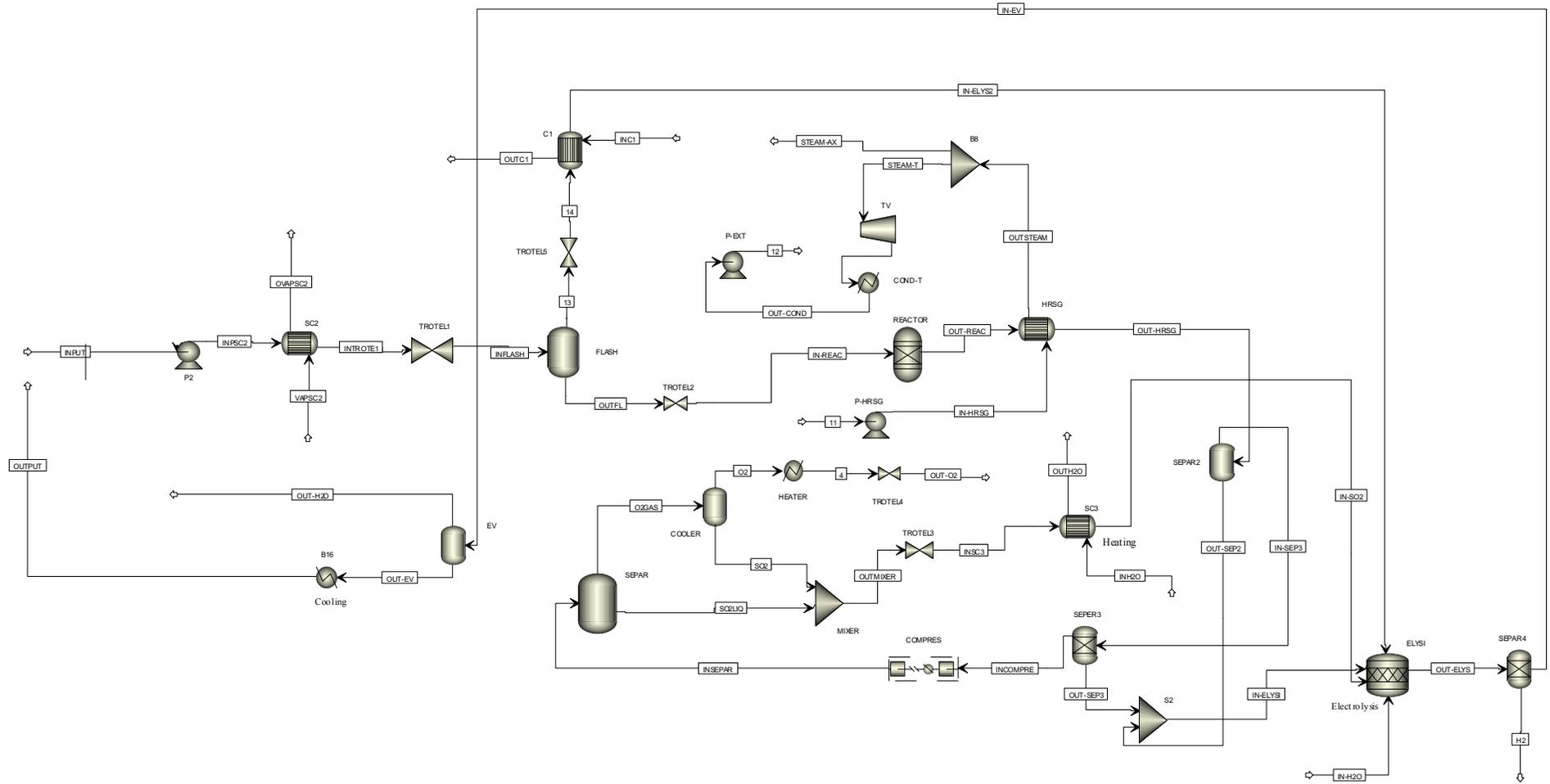
Fig. 5 Simulation of Westinghouse cycle in AspenPlus
