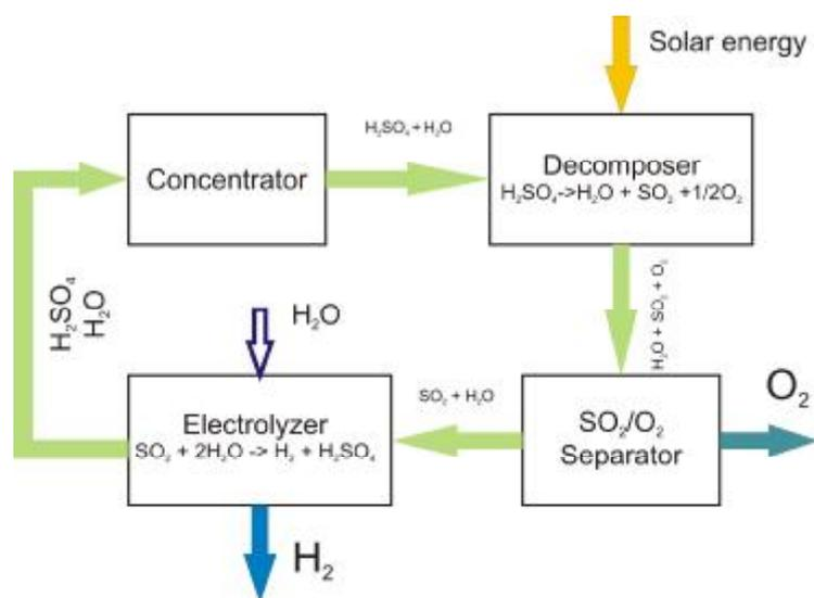
Fig. 2 Westinghouse cycle – simplified model
