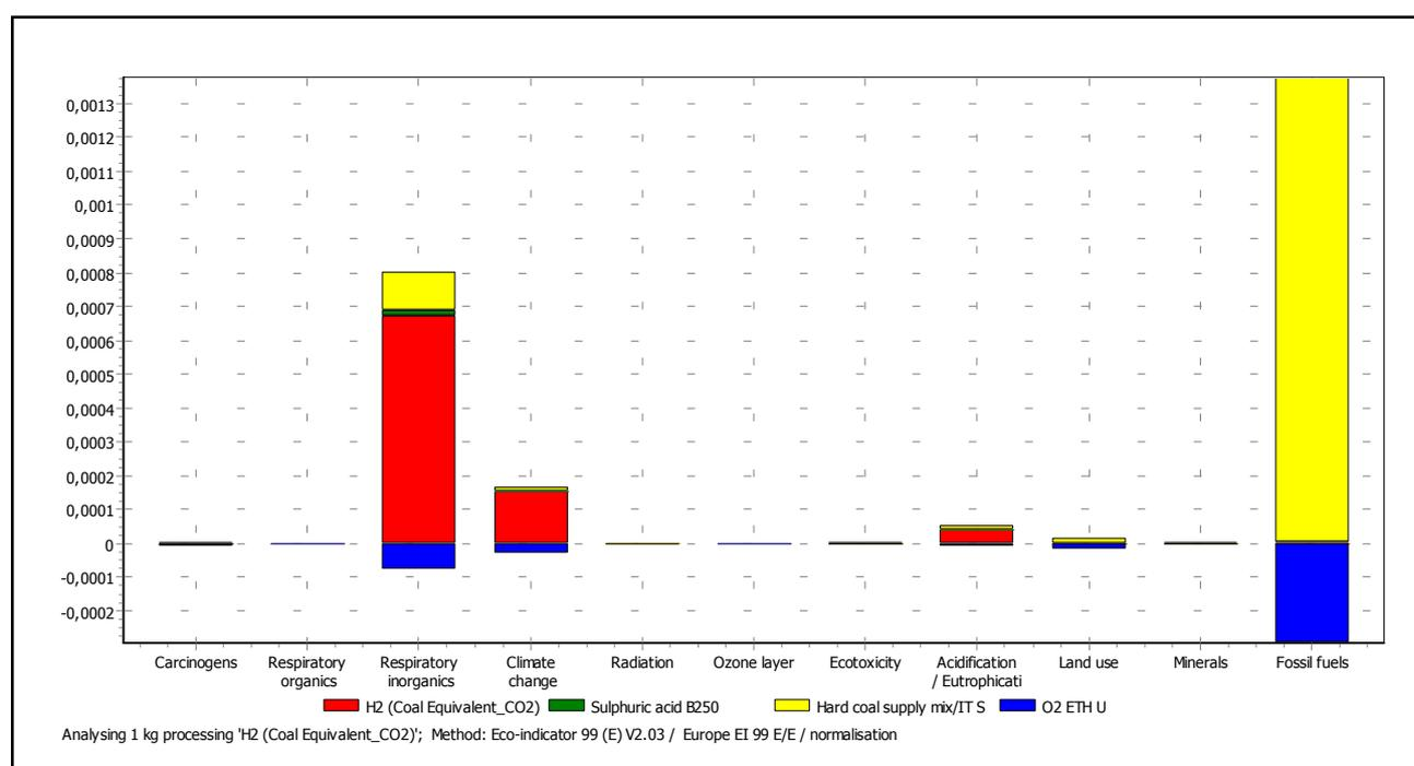
Fig. 8 LCA results (normalized) for  $H_2$  production via Westinghouse cycle
