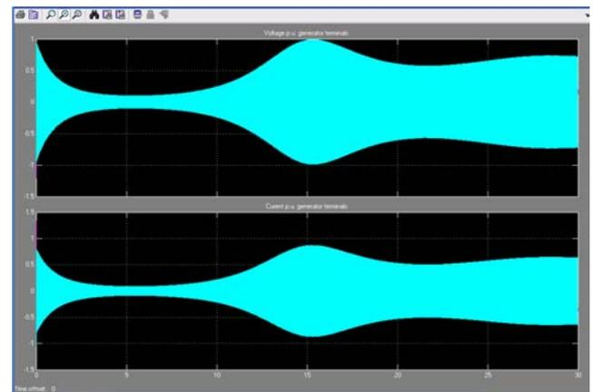
**Fig. 2 Induction generator terminal voltage  $V_L$ , and line current  $I_L$**
