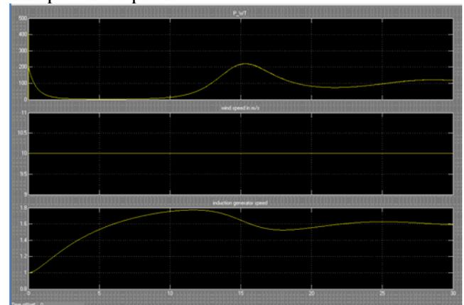
**Fig. 3 Power in KW, wind speed in m/s and induction generator speed in p.u.**
