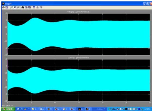
Fig. 4 Induction generator terminal voltage  $V_L$ , and line current  $I_L$
