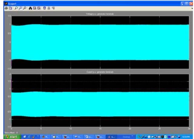
Fig. 6 Induction generator terminal voltage  $V_L$ , and line current  $I_L$
