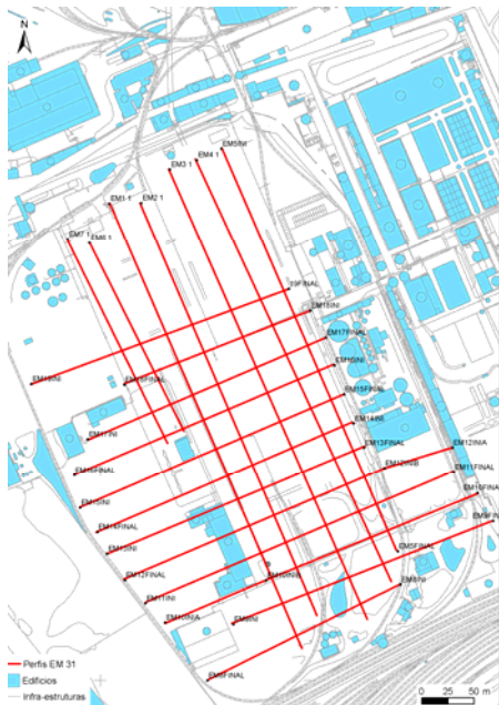
Fig.9 – Geometry of electromagnetic campaign (in [2])
