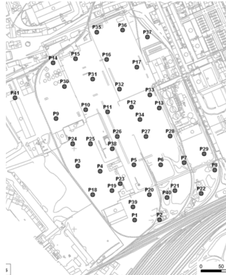
Fig.14 – Field survey: trial pits campaign for soils (in [2])
