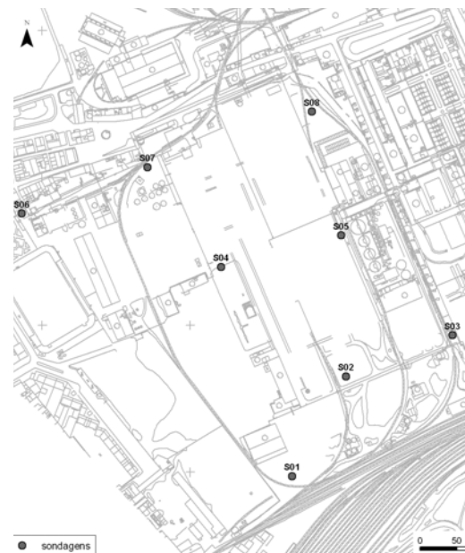
Fig.15 – Field survey :drilling campaign for groundwater (in [2])
