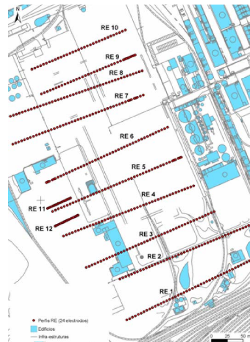
Fig.7 – Resistivity profiles geometry (in [2])
