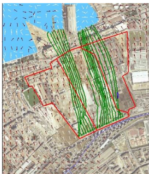
Fig.31 – Dynamics of local groundwater flow and path of a contaminated plume (in [2])
