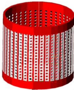
Fig.12 Sketch of anode plate of the fuel cell
