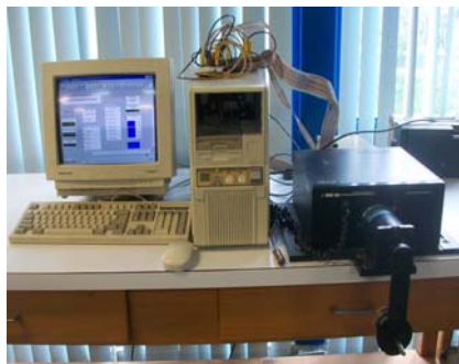
Fig.2 The simple pendulum in closed-loop. Control and Automation Laboratory. Universidad de Los Andes.
