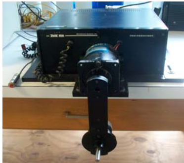
Fig.1 Mechanical system: the simple pendulum. Control and Automation Laboratory. Universidad de Los Andes.
