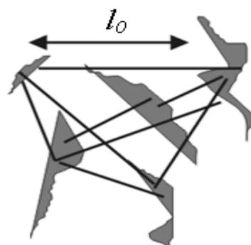
Fig.1 The element of a structured body with an average distance  $l_0$  between pores.
