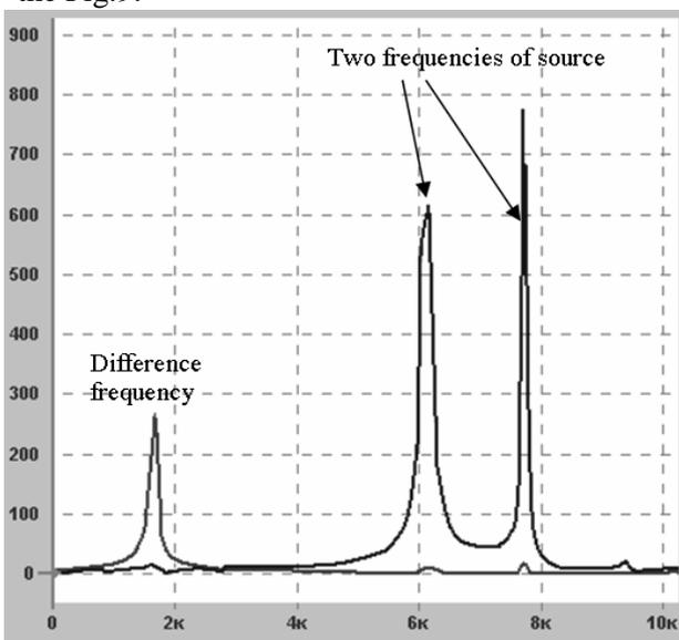
Fig.9 Spectra of quasi-sinusoidal signals. The horizontal axis shows the frequency with step equal 2000Hz. The vertical axis shows the amplitudes. (Egorov G.V. [6])
