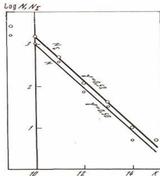
Fig.4 Experimental dependence seismic events numbers versus energy, which is proportional to cracks specific surface. Tangent of the angle  $\gamma = 0.5 - 0.52$
