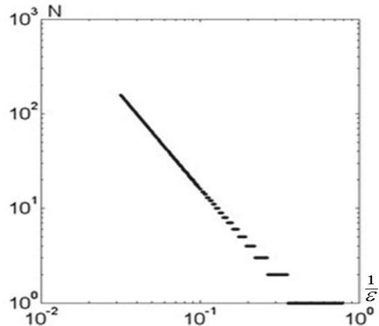
Fig.3 Theoretical dependence of instable events number from cracks specific surface. Tangent of the angle  $\gamma = 0.5$ . It is clearly visible non-uniqueness of solutions with the great energies
