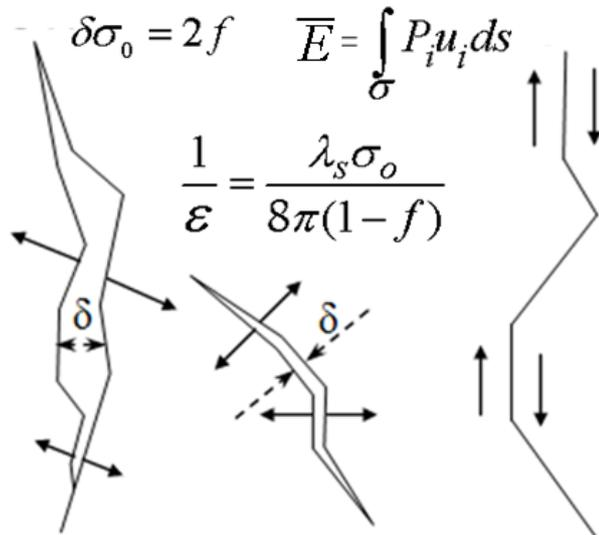
Fig.5 Real shear cracking process (right hand) without of sufficient crack opening corresponds to Richter-Gutenberg law
