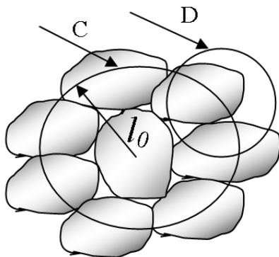
Fig.2 The problem of creation of equilibrium equation into arbitrary element of discrete medium
