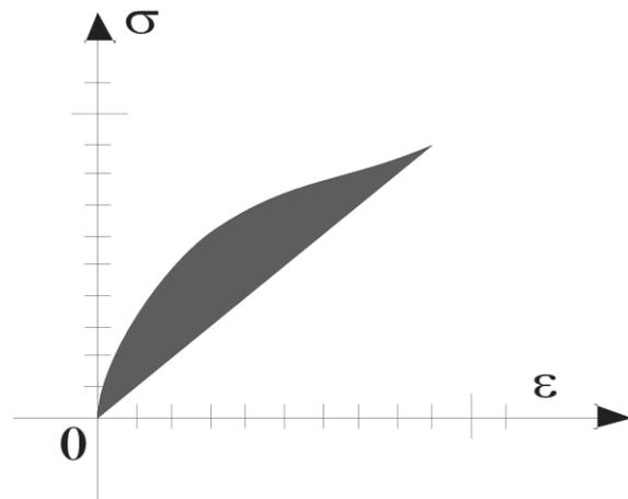
Fig.6 There is relation between stress and strain. The loading part has a positive curvature. The downloading part is a straight line. The area between them is dissipated energy.
