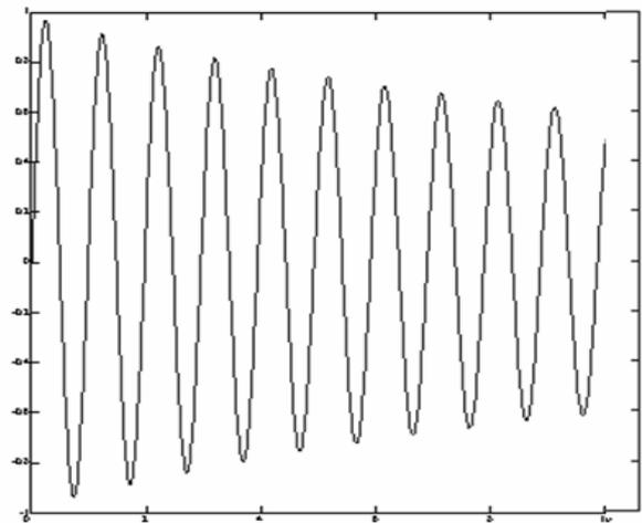
Fig.7 The attenuation of sinusoidal impulse depends on distance. The nonlinear parameter is 0.1. The logarithmic decrement is almost constant value.
