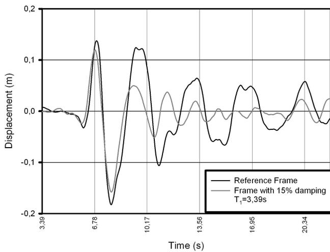
Fig. 19 Displacements - reference frame versus frame with 15% damping (VRANCEA)
