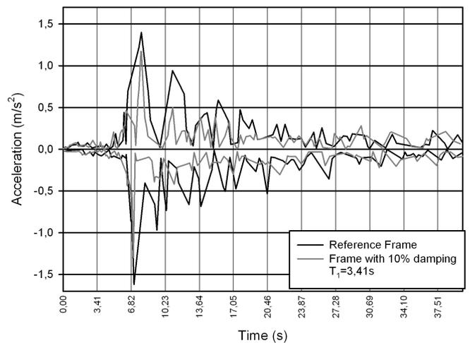
Fig. 36 Acceleration mitigation curves - reference frame versus frame with 10% damping (VRANCEA)
