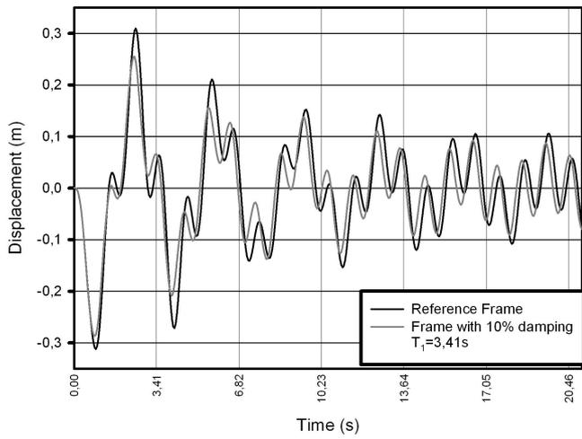
Fig. 9 Displacements - reference frame versus frame with 10% damping (Sinusoidal)
