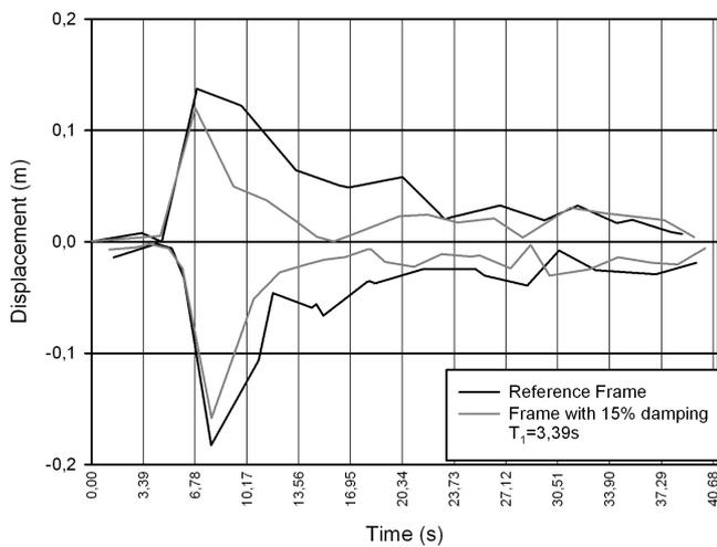
Fig. 25 Displacement mitigation curves - reference frame versus frame with 15% damping (VRANCEA)
