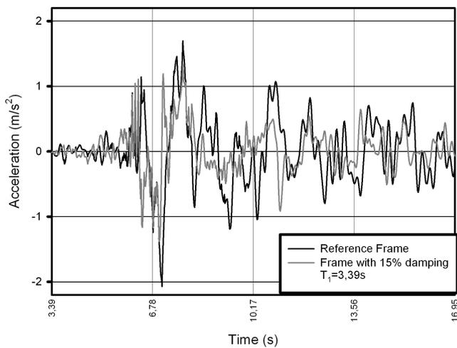
Fig. 43 Acceleration - reference frame versus frame with 15% damping (VRANCEA)
