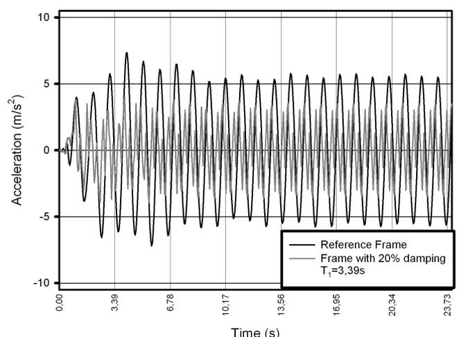
Fig. 47 Acceleration - reference frame versus frame with 20% damping (Sinusoidal)
