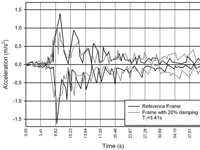
Fig. 38 Acceleration mitigation curves - reference frame versus frame with 20% damping (VRANCEA)
