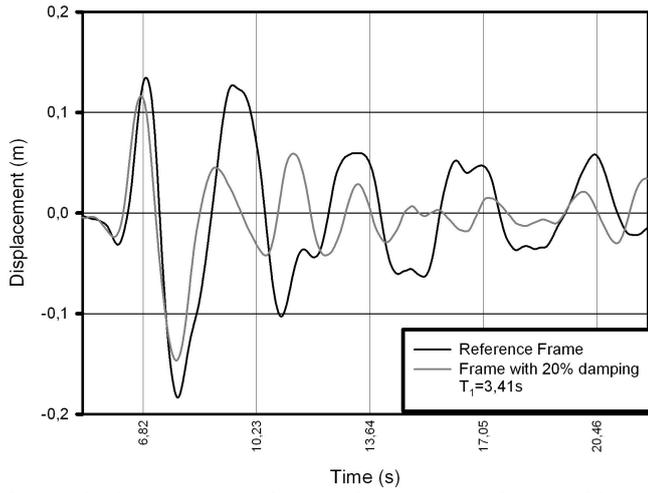
Fig. 8 Displacements - reference frame versus frame with 20% damping (VRANCEA)
