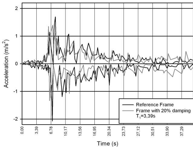
Fig. 50 Acceleration mitigation curves - reference frame versus frame with 20% damping (VRANCEA)
