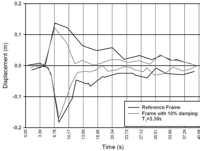
Fig. 24 Displacement mitigation curves - reference frame versus frame with 10% damping (VRANCEA)
