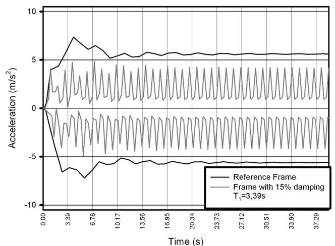
Fig. 52 Acceleration mitigation curves - reference frame versus frame with 15% damping (sinusoidal)
