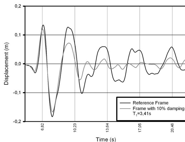
Fig. 6 Displacements - reference frame versus frame with 10% damping (VRANCEA)
