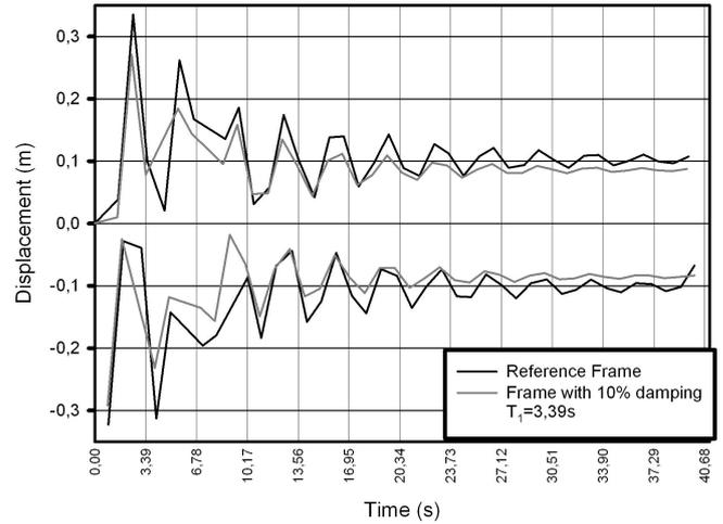
Fig. 27 Displacement mitigation curves - reference frame versus frame with 10% damping (sinusoidal)
