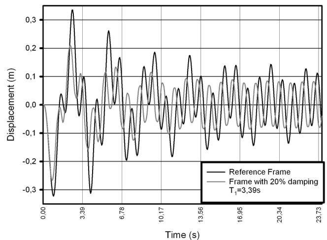
Fig. 23 Displacements - reference frame versus frame with 20% damping (Sinusoidal)
