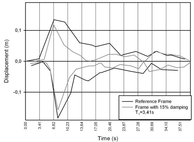
Fig. 13 Displacement mitigation curves - reference frame versus frame with 15% damping (VRANCEA)
