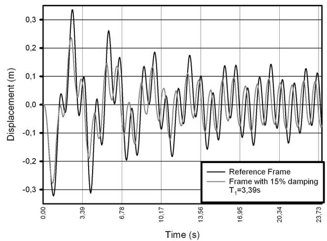
Fig. 22 Displacements - reference frame versus frame with 15% damping (Sinusoidal)
