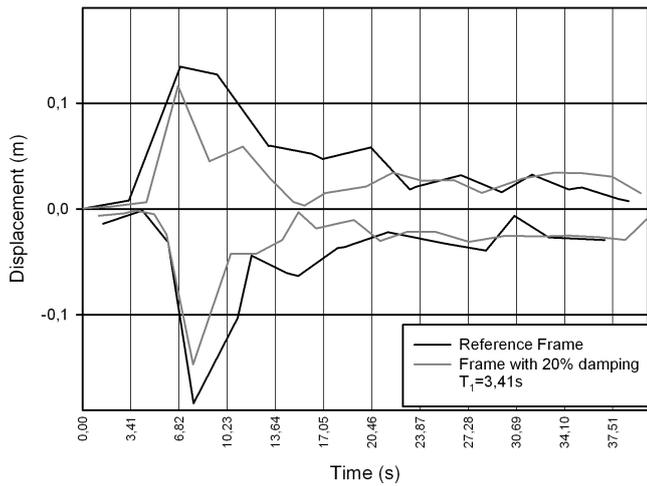
Fig. 14 Displacement mitigation curves - reference frame versus frame with 20% damping (VRANCEA)
