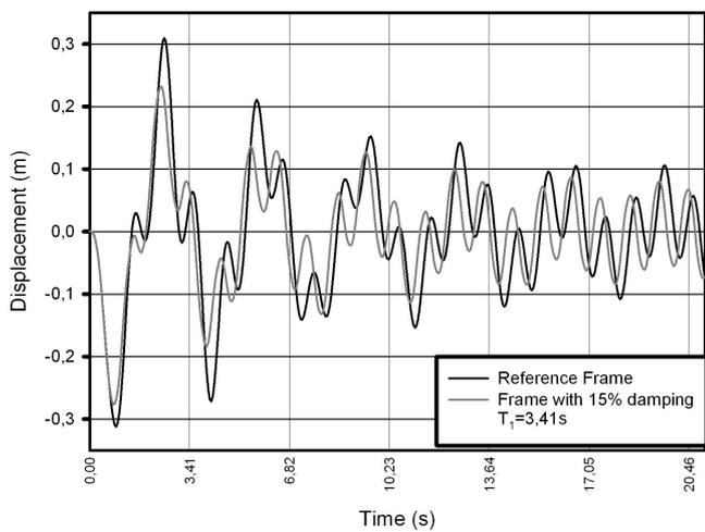
Fig. 10 Displacements - reference frame versus frame with 15% damping (Sinusoidal)
