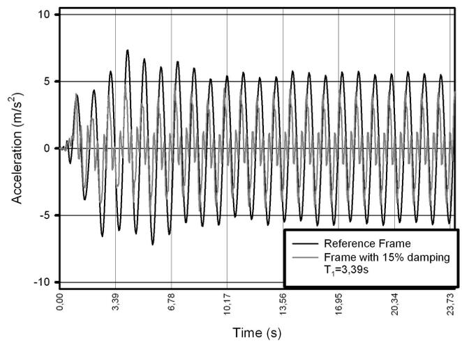
Fig. 46 Acceleration - reference frame versus frame with 15% damping (Sinusoidal)
