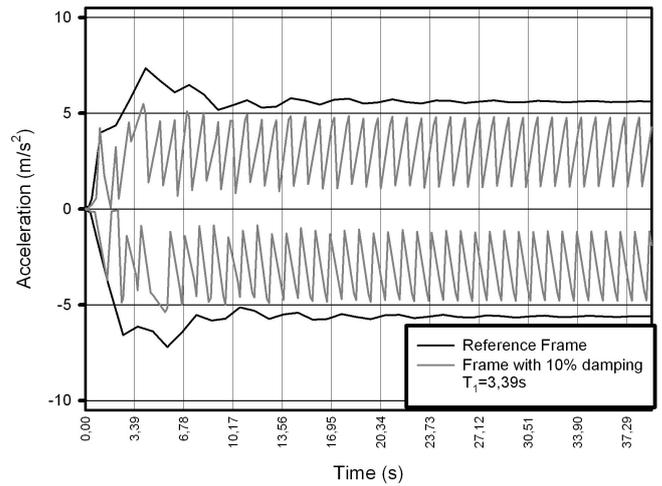
Fig. 45 Acceleration - reference frame versus frame with 10% damping (Sinusoidal)
