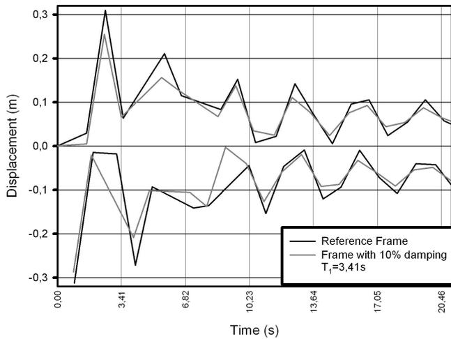
Fig. 15 Displacement mitigation curves - reference frame versus frame with 10% damping (sinusoidal)
