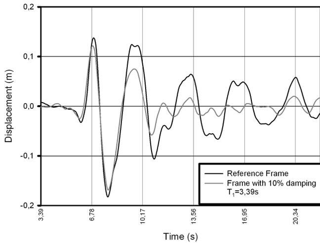
Fig. 18 Displacements - reference frame versus frame with 10% damping (VRANCEA)
