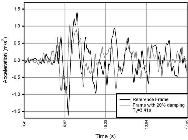
Fig. 32 Acceleration - reference frame versus frame with 20% damping (VRANCEA)
