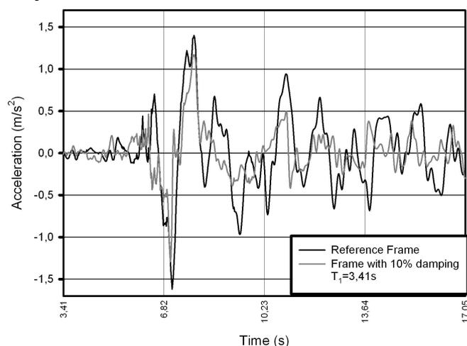
Fig. 30 Acceleration - reference frame versus frame with 10% damping (VRANCEA)
