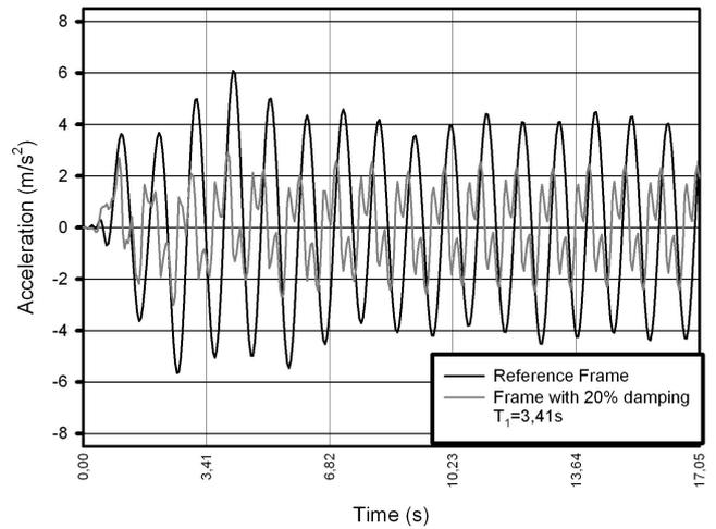
Fig. 35 Acceleration - reference frame versus frame with 20% damping (Sinusoidal)
