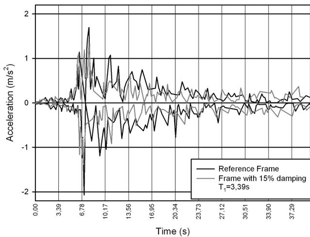
Fig. 49 Acceleration mitigation curves - reference frame versus frame with 15% damping (VRANCEA)
