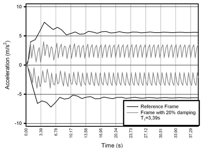
Fig. 53 Acceleration mitigation curves - reference frame versus frame with 20% damping (sinusoidal)
