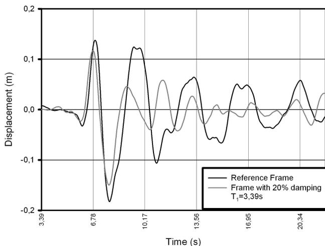
Fig. 20 Displacements - reference frame versus frame with 20% damping (VRANCEA)
