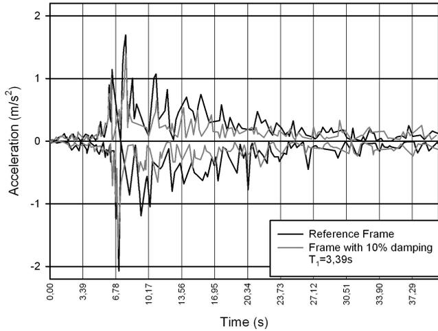
Fig. 48 Acceleration mitigation curves - reference frame versus frame with 10% damping (VRANCEA)
