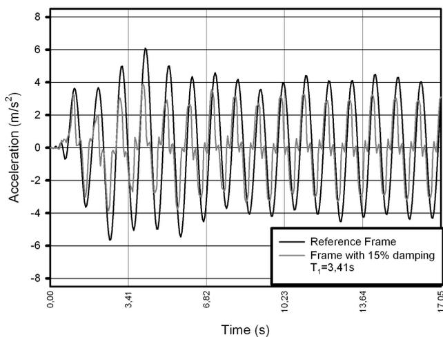
Fig. 34 Acceleration - reference frame versus frame with 15% damping (Sinusoidal)
