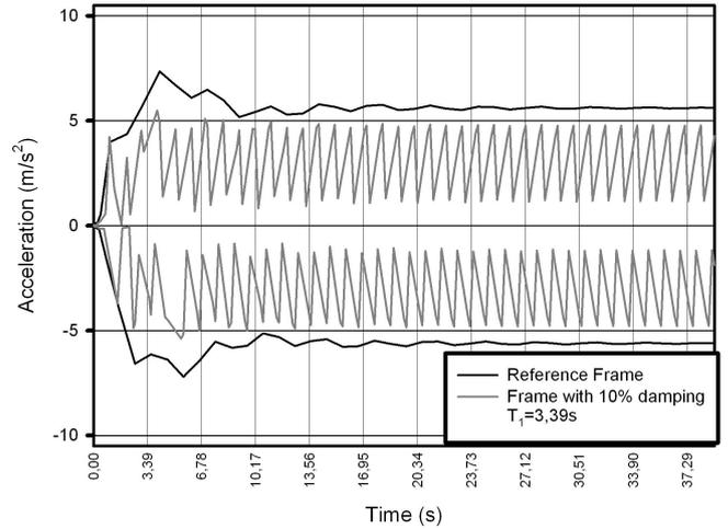
Fig. 51 Acceleration mitigation curves - reference frame versus frame with 10% damping (sinusoidal)
