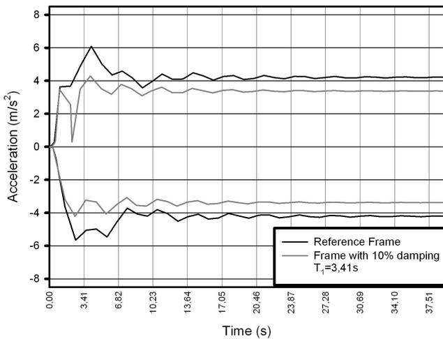
Fig. 39 Acceleration mitigation curves - reference frame versus frame with 10% damping (sinusoidal)
