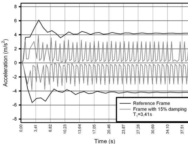
Fig. 40 Acceleration mitigation curves - reference frame versus frame with 15% damping (sinusoidal)
