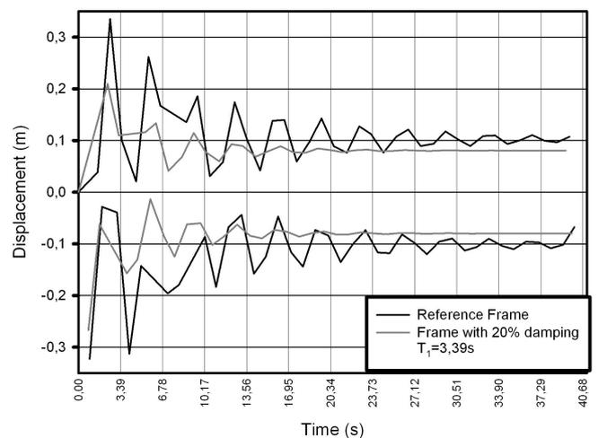
Fig. 29 Displacement mitigation curves - reference frame versus frame with 20% damping (sinusoidal)
