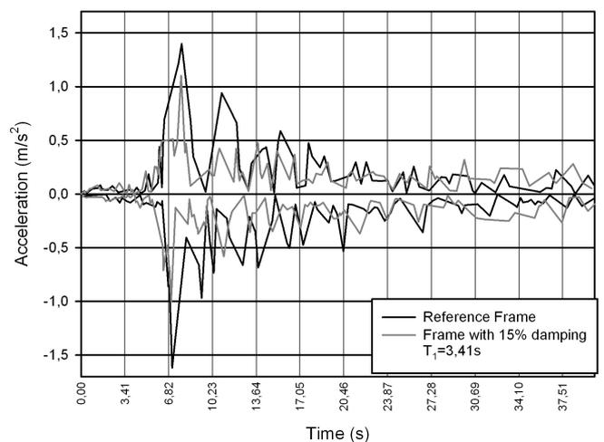
Fig. 37 Acceleration mitigation curves - reference frame versus frame with 15% damping (VRANCEA)
