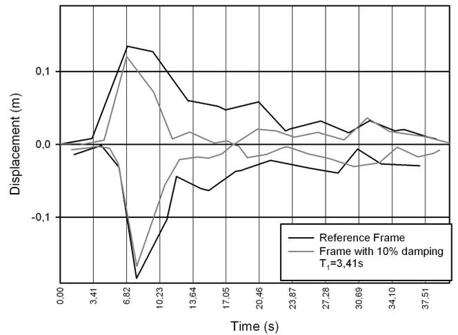
Fig. 12 Displacement mitigation curves - reference frame versus frame with 10% damping (VRANCEA)
