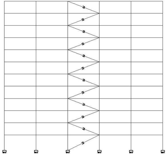
Fig.3 Frame with viscous dampers
