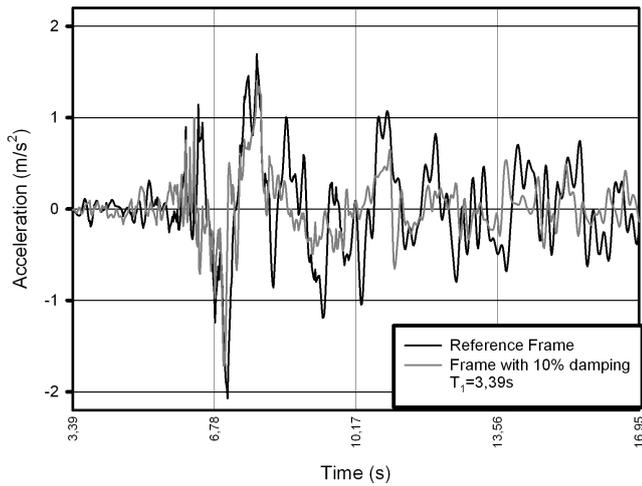
Fig. 42 Acceleration - reference frame versus frame with 10% damping (VRANCEA)
