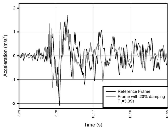
Fig. 44 Acceleration - reference frame versus frame with 20% damping (VRANCEA)
