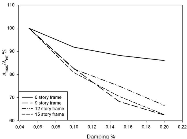
Fig. 61 Damping reduction curves positive values (sinusoidal)
