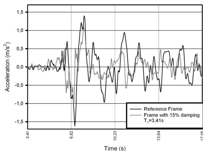
Fig. 31 Acceleration - reference frame versus frame with 15% damping (VRANCEA)
