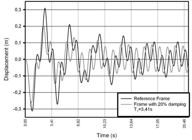
Fig. 11 Displacements - reference frame versus frame with 20% damping (Sinusoidal)
