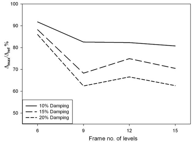
Fig. 57 Damping reduction curves positive values (sinusoidal)
