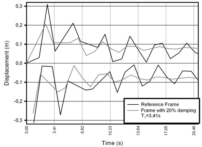
Fig. 17 Displacement mitigation curves - reference frame versus frame with 20% damping (sinusoidal)
