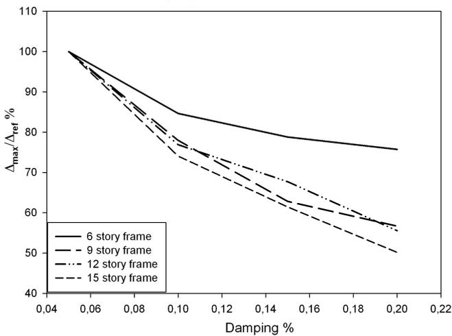
Fig. 60 Damping reduction curves negative values (sinusoidal)
