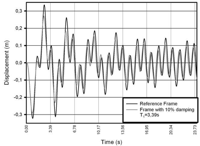
Fig. 21 Displacements - reference frame versus frame with 10% damping (Sinusoidal)
