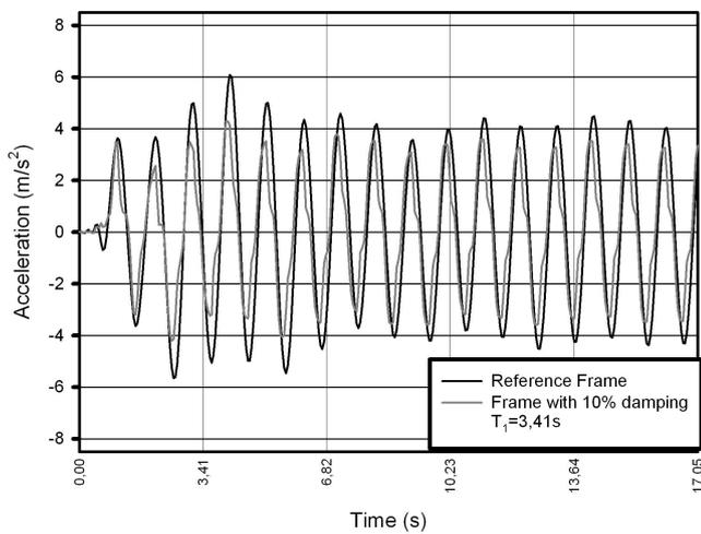
Fig. 33 Acceleration - reference frame versus frame with 10% damping (Sinusoidal)
