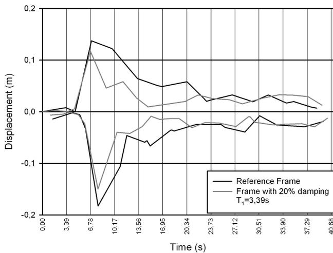
Fig. 26 Displacement mitigation curves - reference frame versus frame with 20% damping (VRANCEA)
