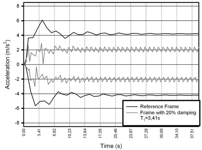
Fig. 41 Acceleration mitigation curves - reference frame versus frame with 20% damping (sinusoidal)
