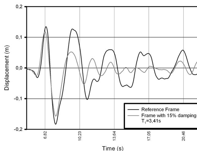
Fig. 7 Displacements - reference frame versus frame with 15% damping (VRANCEA)
