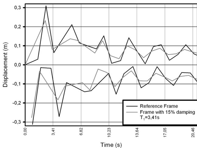
Fig. 16 Displacement mitigation curves - reference frame versus frame with 15% damping (sinusoidal)
