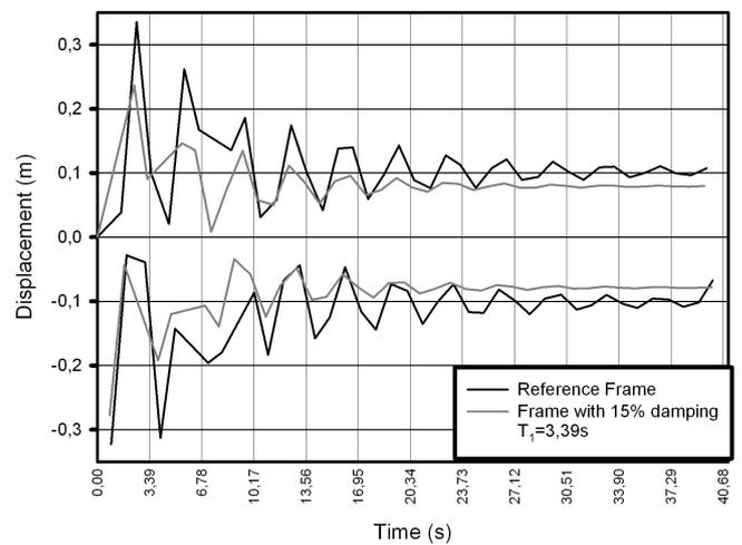
Fig. 28 Displacement mitigation curves - reference frame versus frame with 15% damping (sinusoidal)
