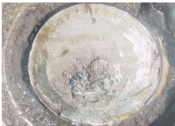
Figure 1. Broken tank wagon axle from a severe derailment, [1].
