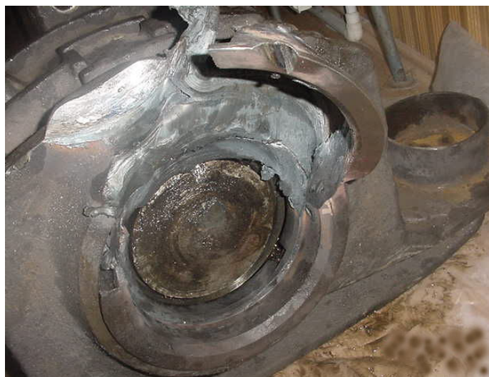
Figure 7. The fracture of bearing box as a result of heat dissipated from friction against the locking ring.
