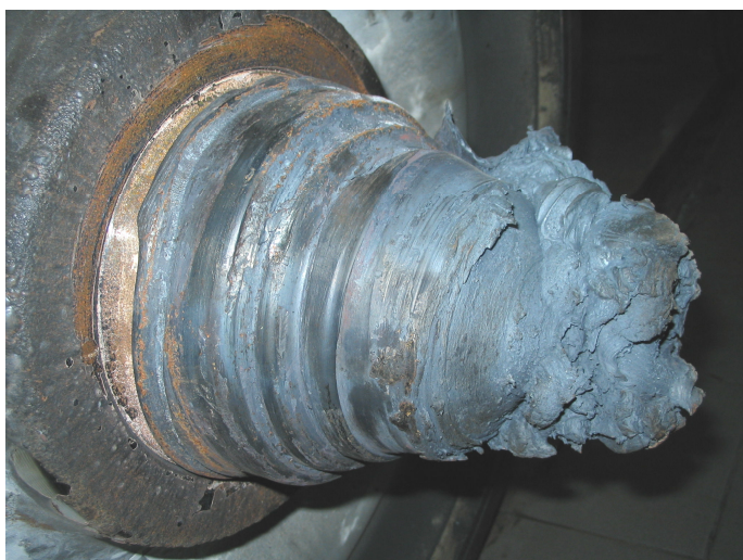
Figure 3. View of end cap and remaining portion of axle stub [3].
