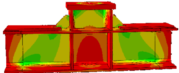
Fig.11 Stresses S_{yy} for strengthened connection
