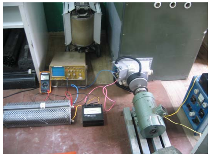
Fig. 5. The generator parameters identification on experimental stand
