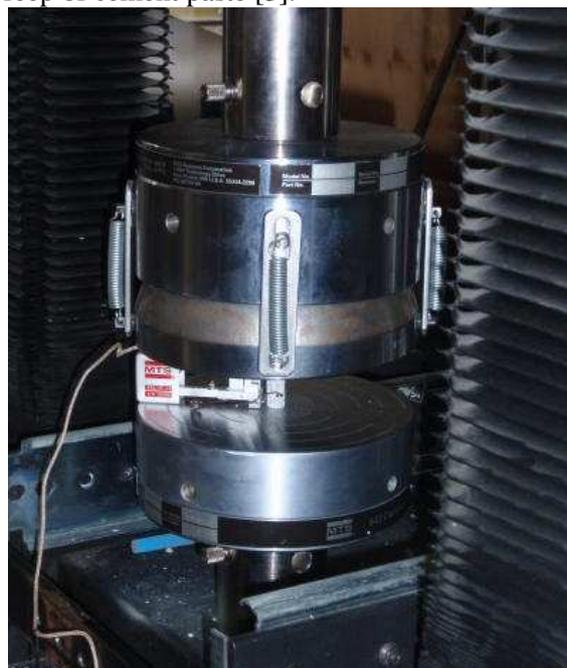
Fig.2: Specimens in compression test equipment.
