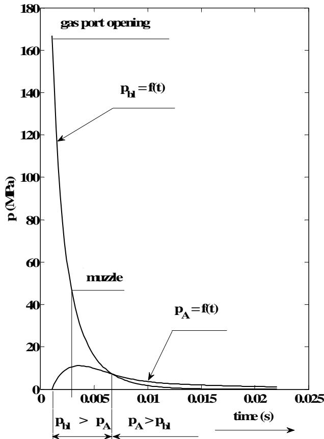
Fig. 5 Gas pressure in cylinder and barrel
