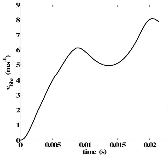
Fig. 11 Breech block carrier velocity
