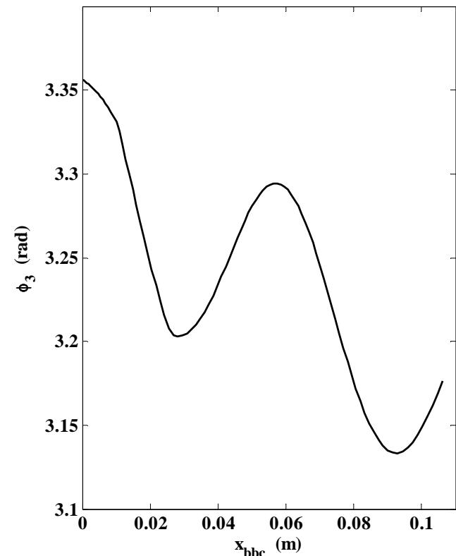
Fig. 13 Connecting rod angle  $\phi_3$
