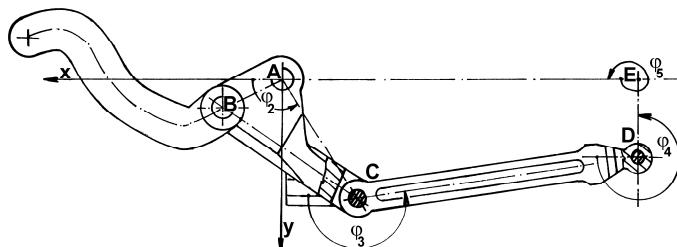
Fig. 2 Eccentric crank mechanism of weapon
