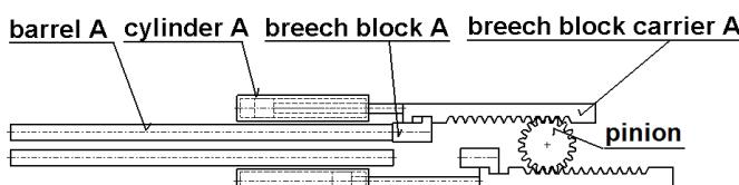
Fig. 1 Principle of design features
