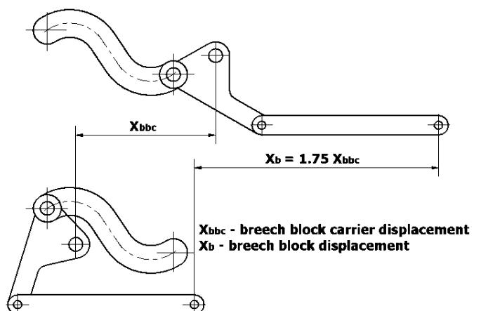
Fig. 14 Explanation of breech block and breech block carrier displacements
