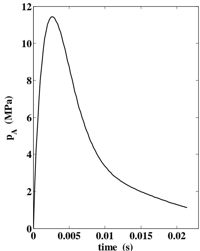
Fig. 17 Gas pressure in gas cylinder
