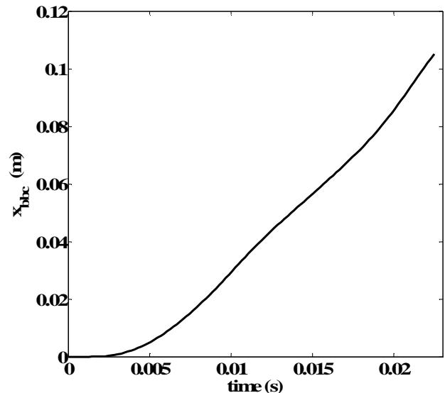
Fig. 10 Breech block carrier displacement
