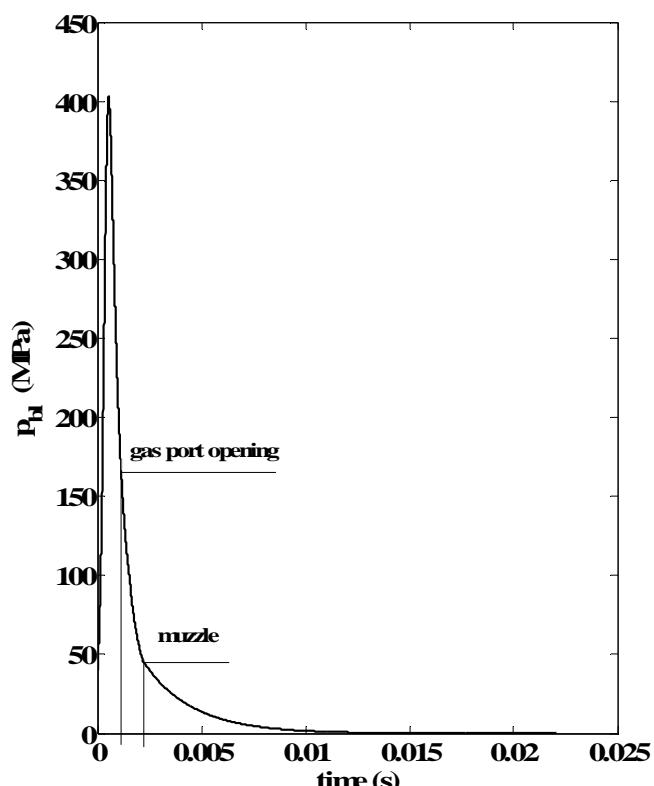
Fig. 4 Pressure in the barrel – cartridge 20x102mm
