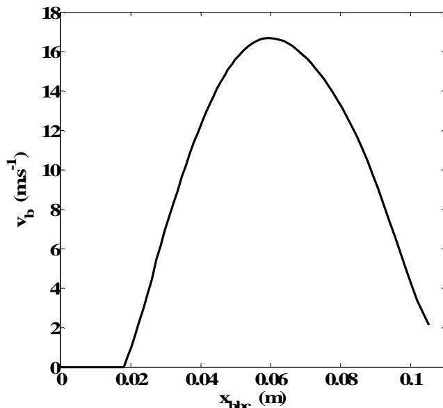
Fig. 15 Breech block velocity
