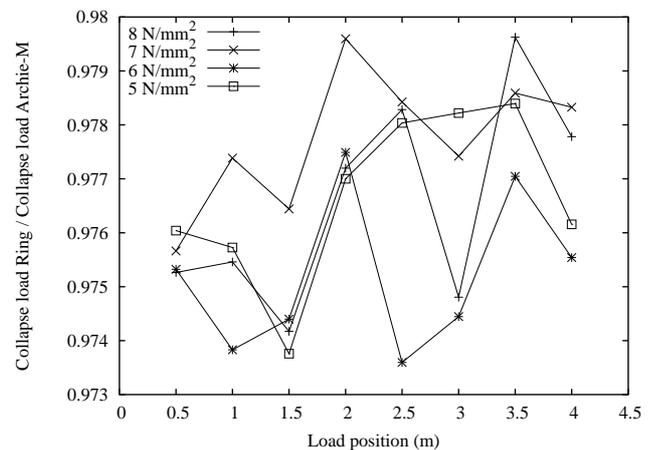
Graph 3: Collapse load ratio for different positions and crushing strength
