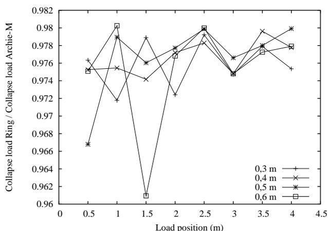
Graph 4: Collapse load ratio for different positions and thickness
