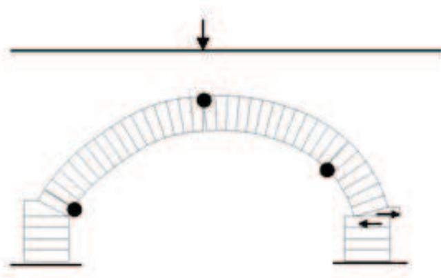
Figure 2: Combined shear-hinge mechanism
