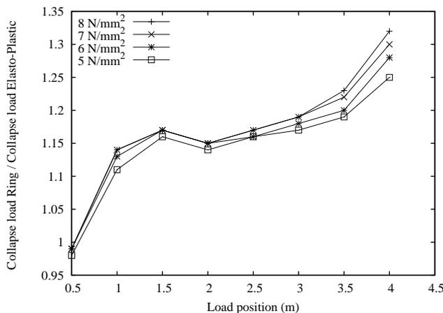
Graph 1: Collapse load ratio for different positions and crushing strength
