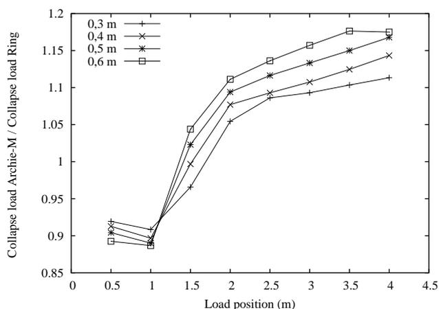
Graph 7: Collapse load ratio for different positions and thickness (Distributed live load)
