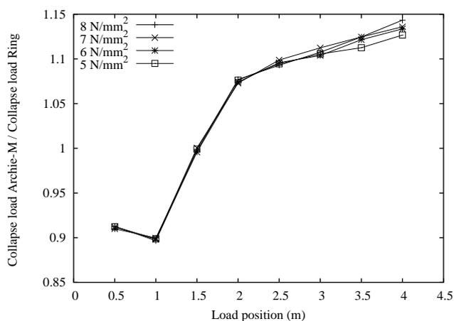
Graph 6: Collapse load ratio for different positions and crushing strength (Distributed live load)
