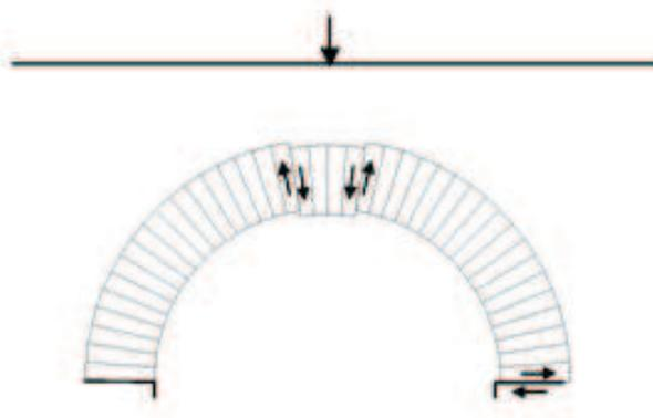
Figure 1: Shear mechanism
