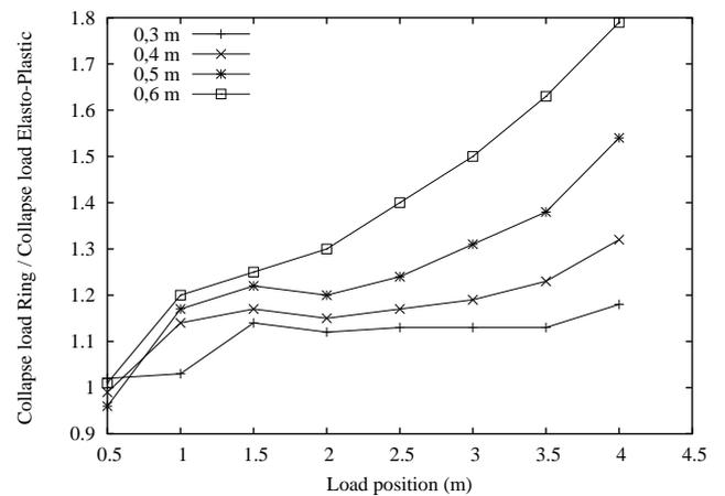
Graph 2: Collapse load ratio for different positions and thickness
