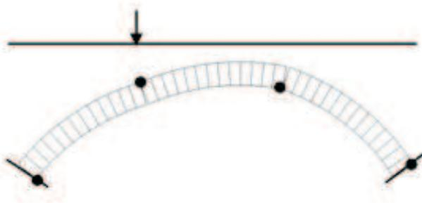
Figure 3: Hinge mechanism
