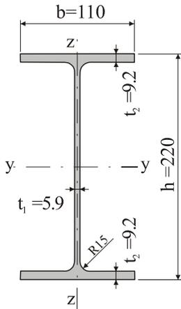
Fig.4 IPE220 Cross section dimensions
