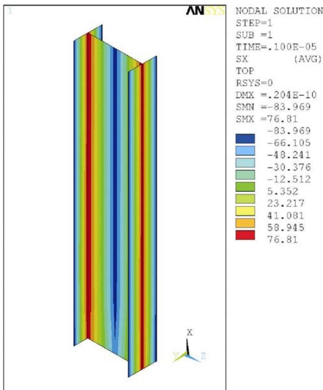
Fig.8 Model of residual stress
