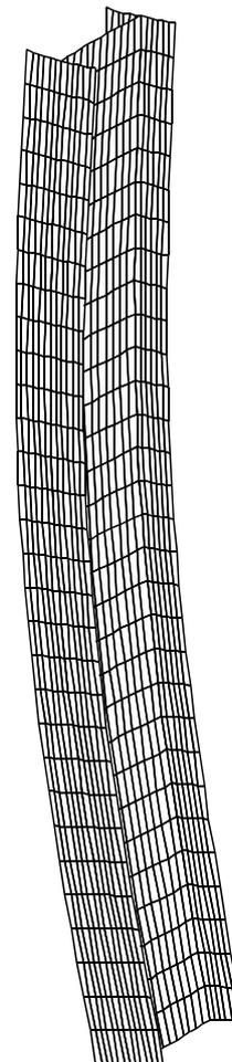
Fig.9 Strut under compression (elements SHELL 181)
