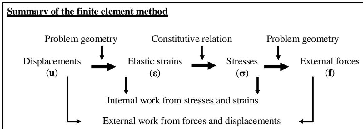
Fig. 2: Summary of the finite element method
