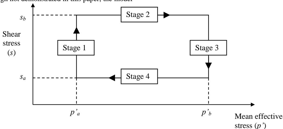
**Fig. 1: Stress path of non-zero area.**
