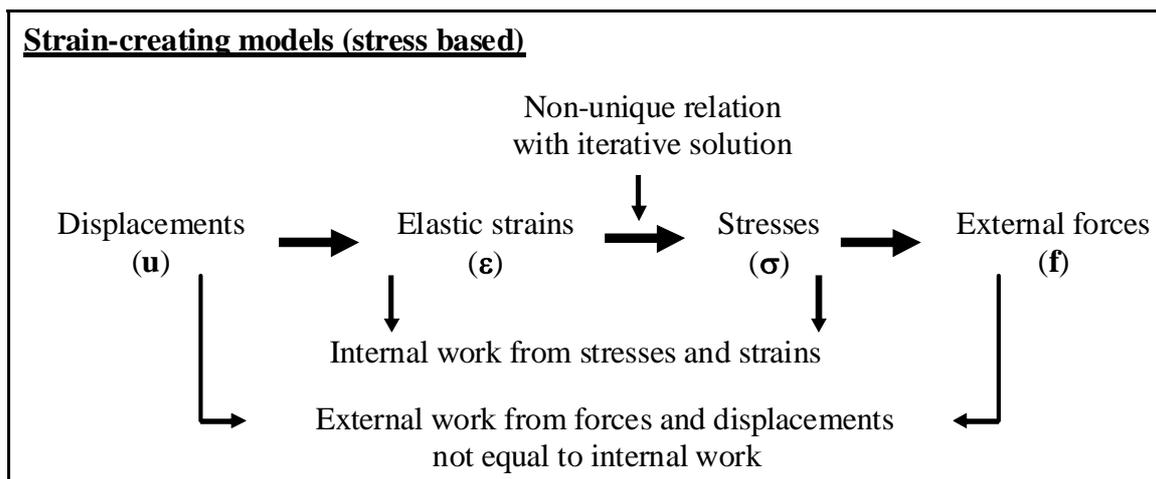
**Fig. 4: Implementation of the finite element method for non-rigorous non-linear elastic models**
