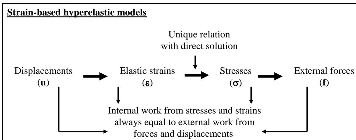
Fig. 6: Implementation of the finite element method for strain-based hyperelastic models
