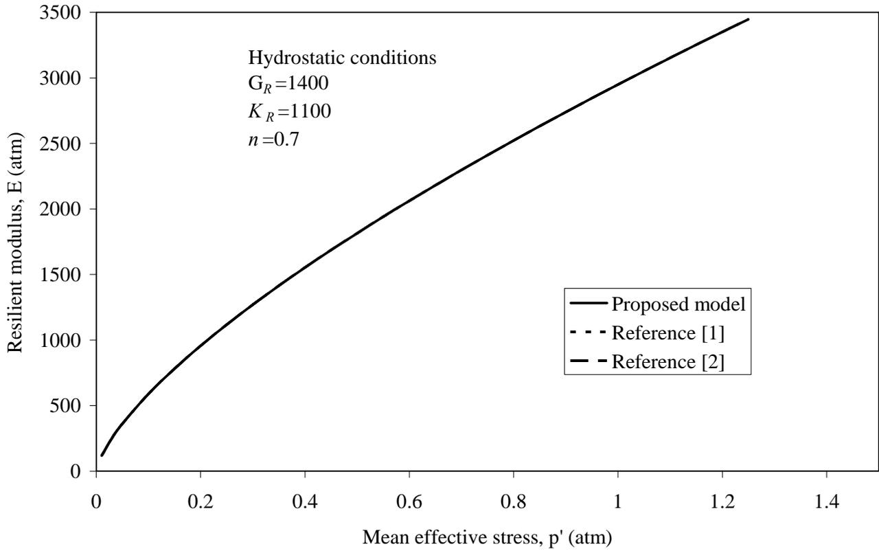
**Fig. 7: Model behaviour under hydrostatic conditions (no shear)**
