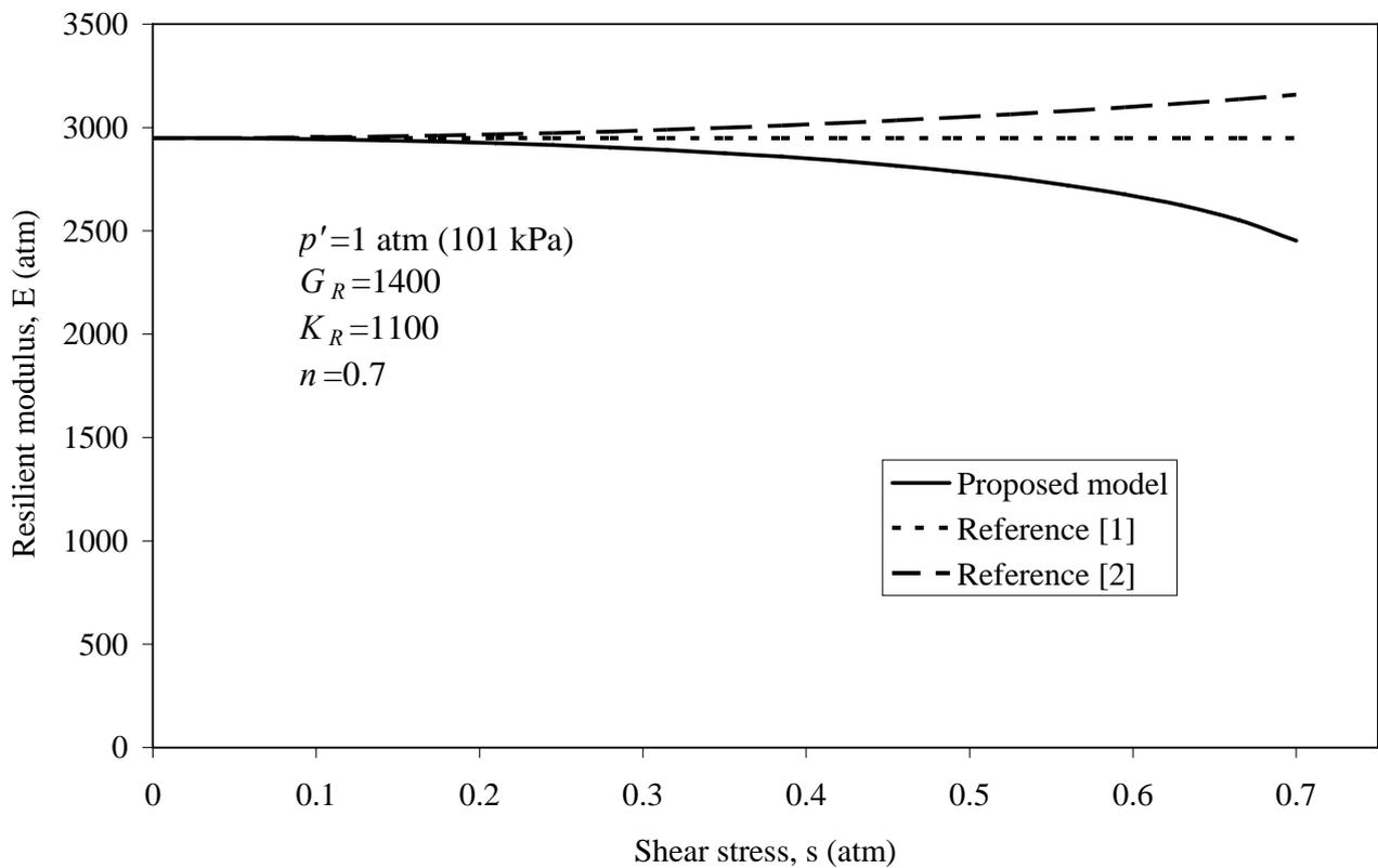
**Fig. 8: Model behaviour under constant mean effective stress**
