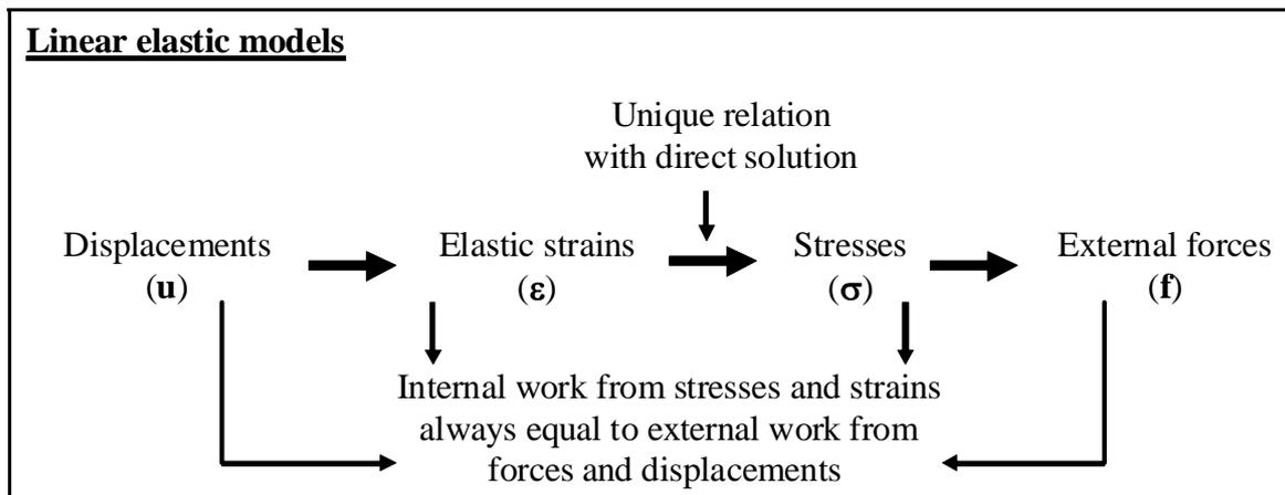
Fig. 3: Implementation of the finite element method for linear elastic models
