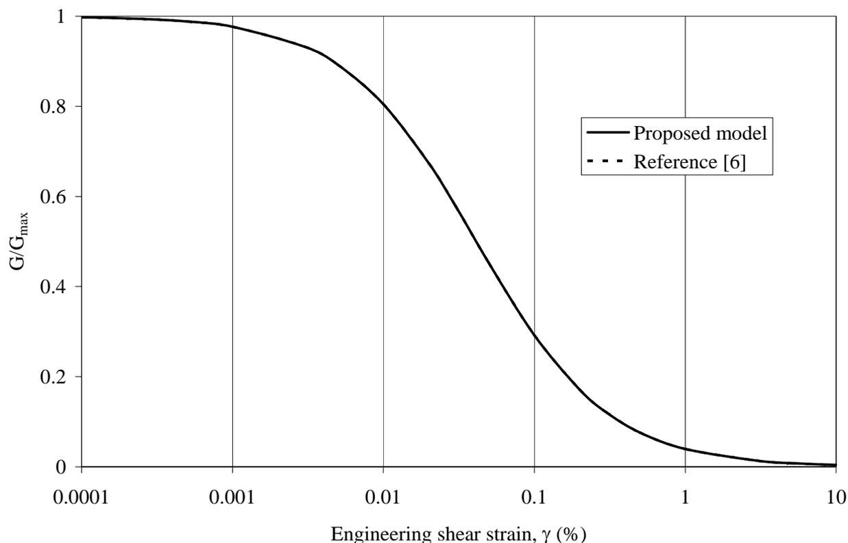
**Fig. 9: Predicted model response when combined with Hardin and Drnevich [6] modulus degradation curve.**
