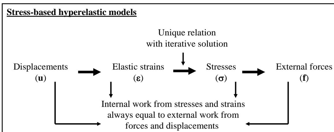
**Fig. 5: Implementation of the finite element method for stress-based hyperelastic models**
