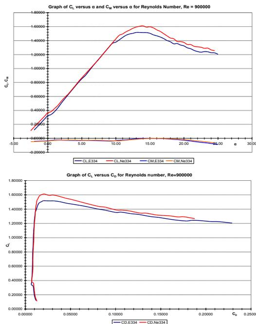
Figure 6b. Graph of comparison between E334 and Ne334 airfoil for  $C_L$  versus  $\alpha$ ,  $C_M$  versus  $\alpha$  and  $C_D$  versus  $C_L$  at Reynolds number of  $0.9 \cdot E^6$
