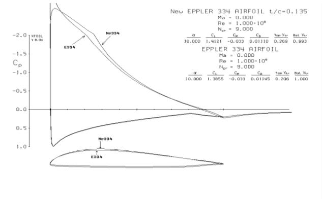
Figure 5d. Graph of pressure distribution over E334 and Ne334 airfoil at  $\alpha = 10^\circ$  at  $Re = 1 * 10^6$
