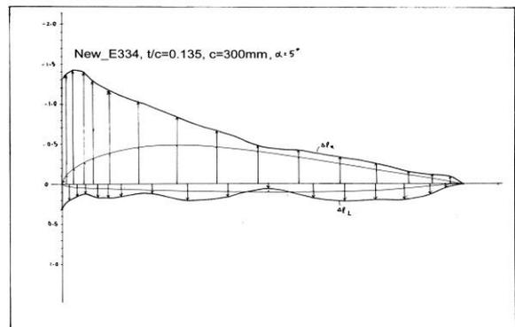
Figure 12c. The pressure distribution of airfoil Ne334 test model at angle of attack,  $\alpha = 5^\circ$ .
