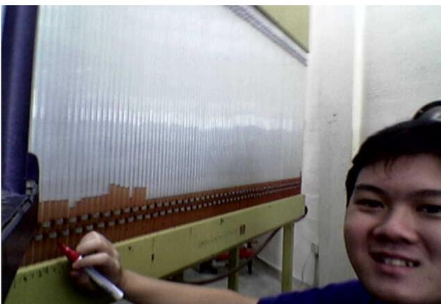
Figure 11. Taking reading from the manometer
