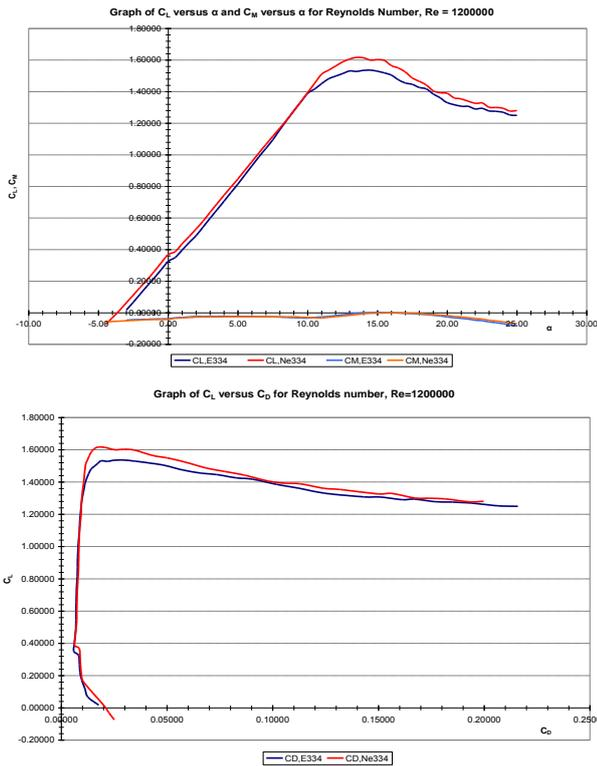
Figure 6e. Graph of comparison between E334 and Ne334 airfoil for  $C_L$  versus  $\alpha$ ,  $C_M$  versus  $\alpha$  and  $C_D$  versus  $C_L$  at Reynolds number of  $1.2 \cdot 10^6$
