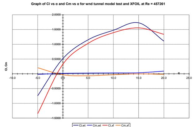
Figure 13. Graph of the comparison between wind tunnel test model (wt) and XFOIL (xf) results for  $C_L$  versus  $\alpha$  and  $C_M$  versus  $C_L$  for Ne334 airfoil at  $R_N = 457,261$
