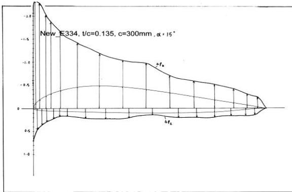
Figure 12e. The pressure distribution of airfoil Ne334 test model at angle of attack,  $\alpha = 15^\circ$ .
