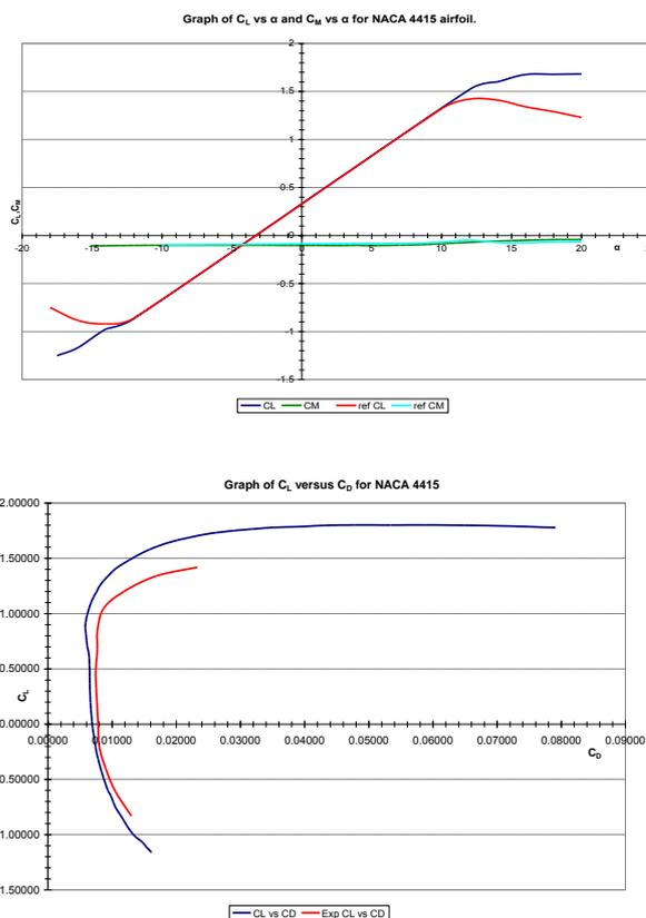
Figure 4. The NACA 4415 airfoil aerodynamic characteristics, both from XFOIL and reference [3] at Re = 3000000
