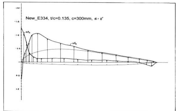
Figure 12b. The pressure distribution of airfoil Ne334 test model at angle of attack,  $\alpha = 0^\circ$ .
