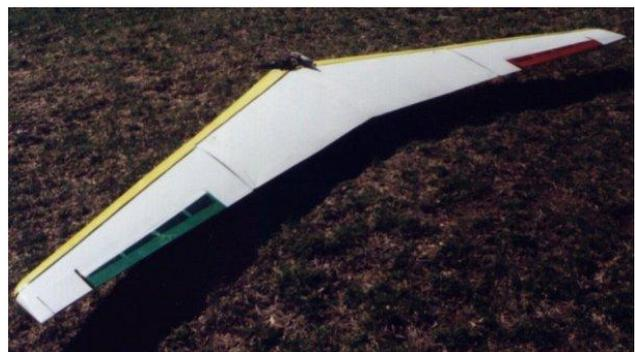
Figure 1. Flying Wing Unmanned Aerial Vehicle.
