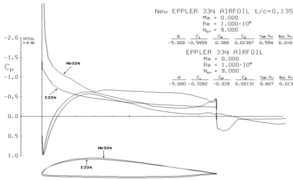
Figure 5a. Graph of pressure distribution over E334 and Ne334 airfoil at  $\alpha = -5$  at  $Re = 1 * 10^6$
