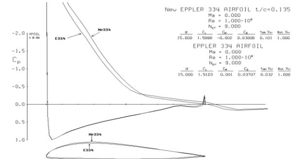
Figure 5e. Graph of pressure distribution over E334 and Ne334 airfoil at  $\alpha = 15^\circ$  at  $Re = 1 * 10^6$
