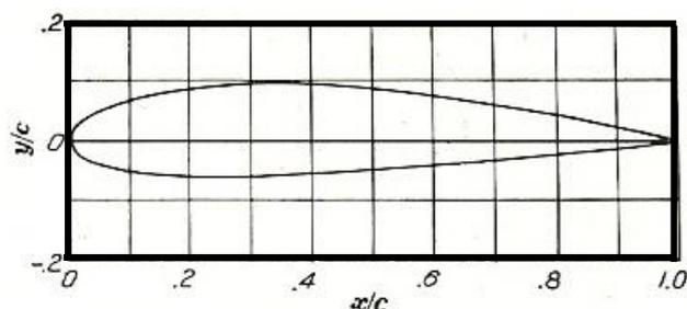
Figure 3. The geometry of NACA 4415 airfoil
