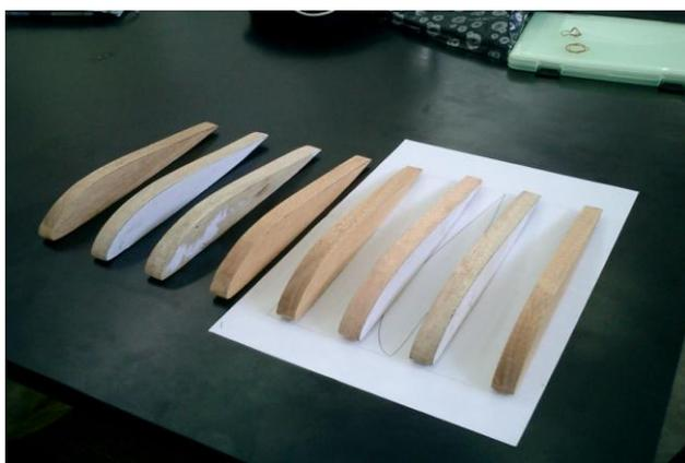
Figure 9b. Airfoil is scale to 30cm of chord
