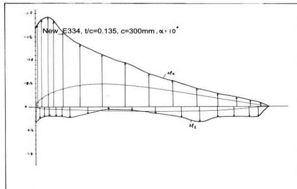
Figure 12d. The pressure distribution of airfoil Ne334 test model at angle of attack,  $\alpha = 10^\circ$ .
