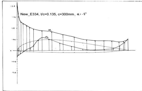
Figure 12a. The pressure distribution of airfoil Ne334 test model at angle of attack,  $\alpha = -5^\circ$ .
