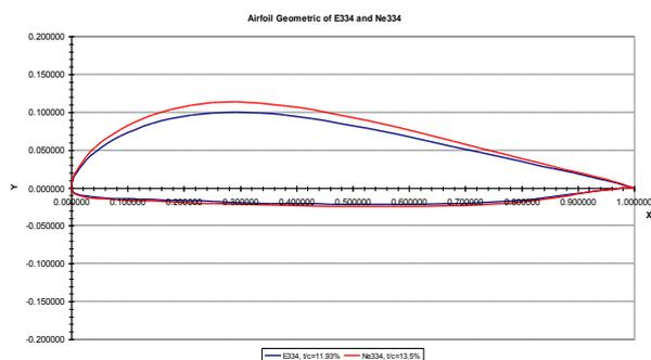
Figure 2. Eppler E334 and new Ne334 airfoil
