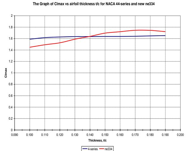
Figure 7. Graph of comparison of NACA 44-series with the new Ne334 for different of thickness
