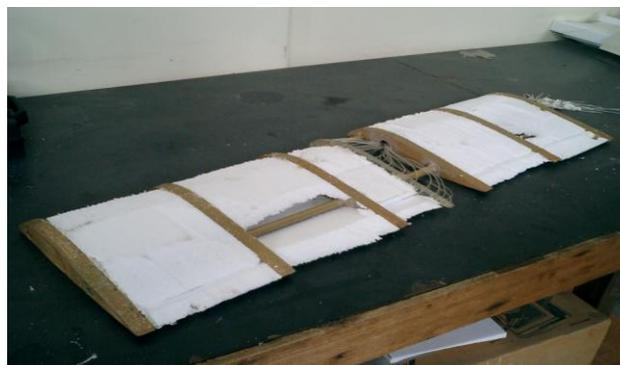
Figure 9f. Final assembly of airfoil model
