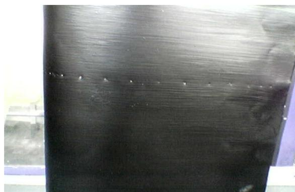
Figure 9g. Flush orifices, there are total of 32 orifices in the test model
