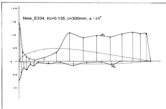
Figure 12f. The pressure distribution of airfoil Ne334 test model at angle of attack,  $\alpha = 20^\circ$ .
