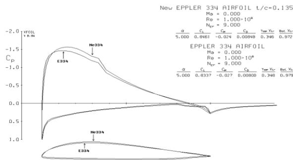
Figure 5c. Graph of pressure distribution over E334 and Ne334 airfoil at  $\alpha = 5^\circ$  at  $Re = 1 * 10^6$
