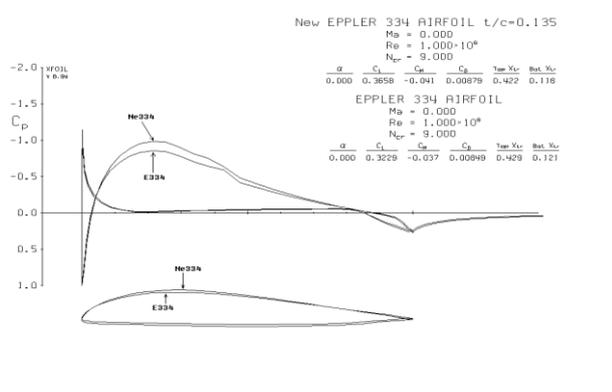
Figure 5b. Graph of pressure distribution over E334 and Ne334 airfoil at  $\alpha = 0^\circ$  at  $Re = 1 * 10^6$
