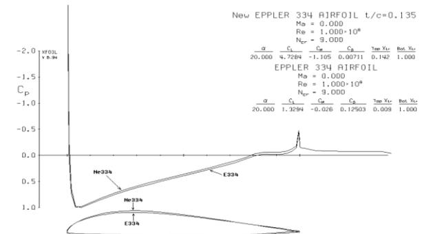
Figure 5f. Graph of pressure distribution over E334 and Ne334 airfoil at  $\alpha = 20^\circ$  at  $Re = 1 * 10^6$
