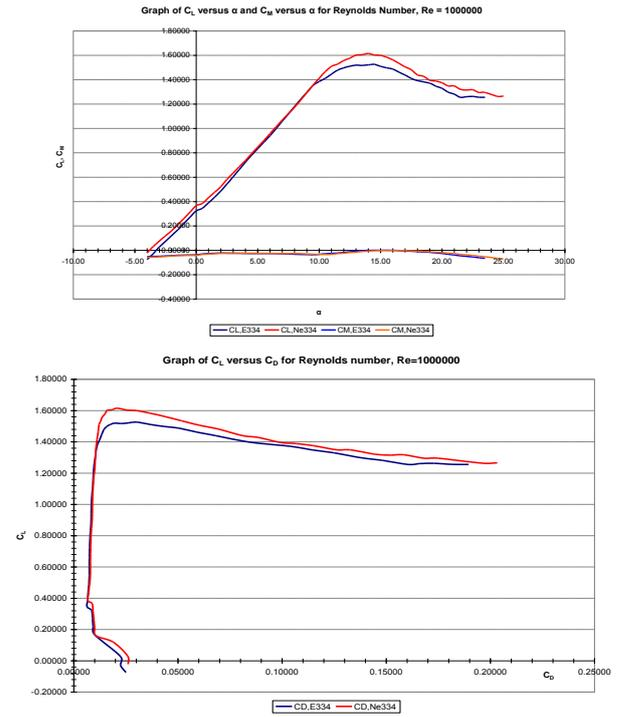
Figure 6c. Graph of comparison between E334 and Ne334 airfoil for  $C_L$  versus  $\alpha$ ,  $C_M$  versus  $\alpha$  and  $C_D$  versus  $C_L$  at Reynolds number of  $1 \cdot E^6$
