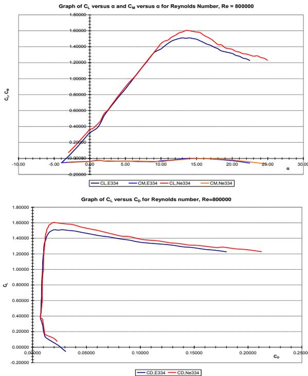
Figure 6a. Graph of comparison between E334 and Ne334 airfoil for  $C_L$  versus  $\alpha$ ,  $C_M$  versus  $\alpha$  and  $C_D$  versus  $C_L$  at Reynolds number of  $0.8 \cdot E^6$
