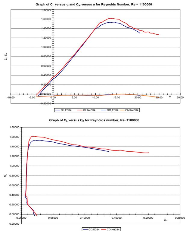
Figure 6d. Graph of comparison between E334 and Ne334 airfoil for  $C_L$  versus  $\alpha$ ,  $C_M$  versus  $\alpha$  and  $C_D$  versus  $C_L$  at Reynolds number of  $1.1 \cdot E^6$
