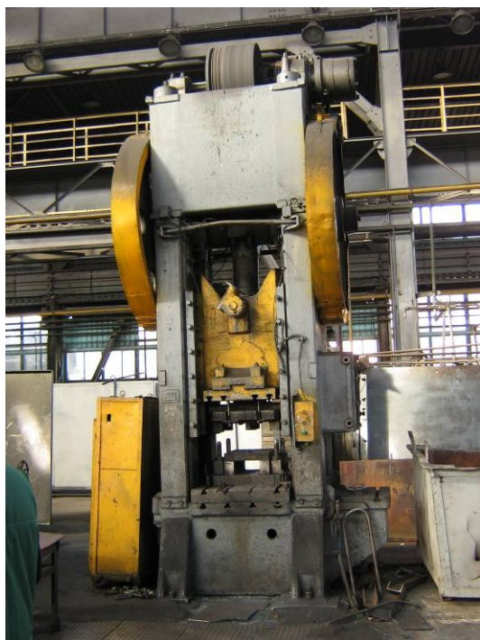
Fig. 2 Press with eccentric
