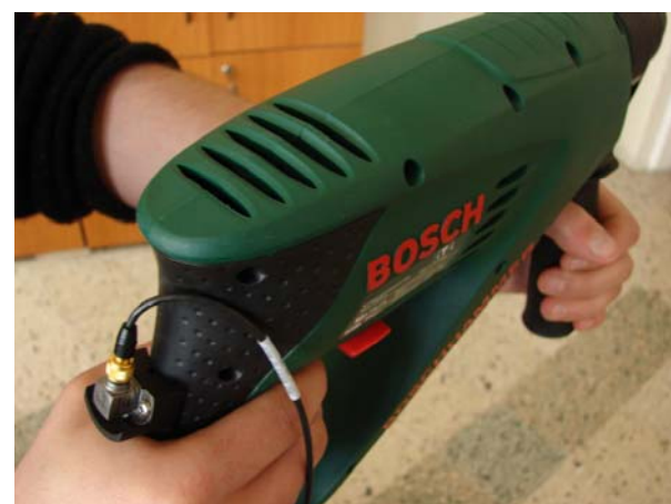
Fig. 8 Example of HAV experimental set-up at Transilvania University of Brasov
