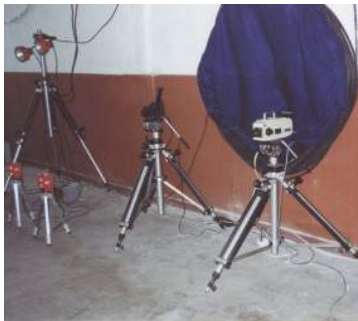
Fig 15. Speed camera and photocells measuring the vehicle's speed
