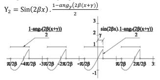
Fig. 24:  $Y_2$  describes the waveform of the thyristor voltage  $v_{T1}$  on the thyristor T1.
