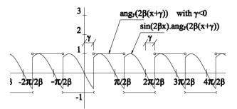
Fig. 23: Y<sub>1</sub> describes the waveform of the single phase bridge fully controlled circuit.
