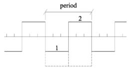
Fig. 17: number of rectangles in the Steprectangular waveform first order (n=1).
