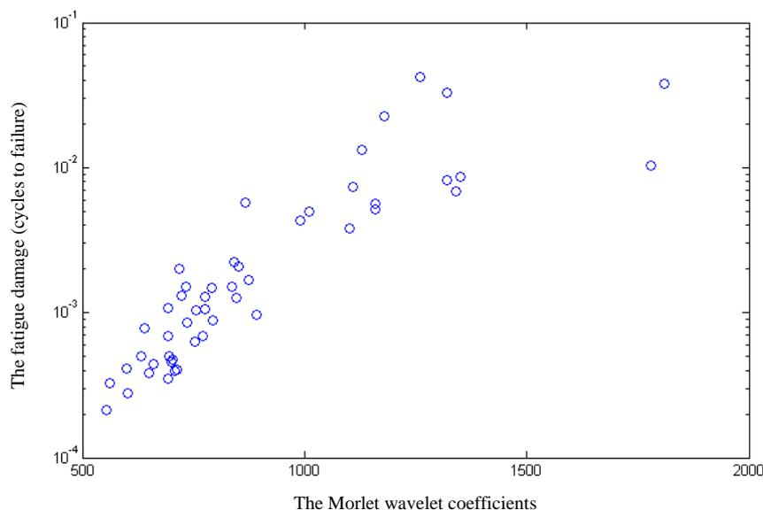
Fig. 5 Scatter plot of the fatigue damage and the Morlet wavelet coefficient
