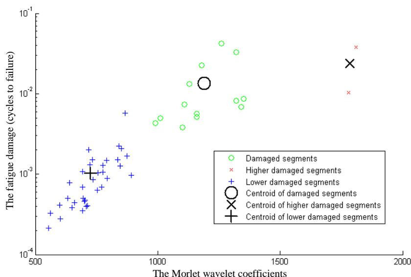
Fig. 6 Clustering of the fatigue damage and the Morlet wavelet coefficient
