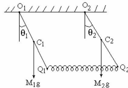
Fig. 1. The coupled pendulum.
