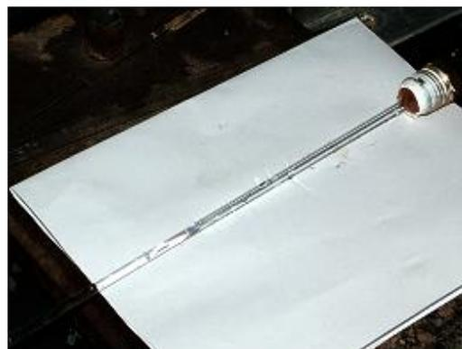
Fig.2. Joint capillary tube/brass conector
