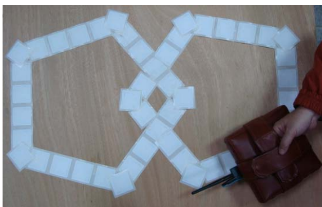
Fig. 9. The situation when the hand tackles with the RFID reader pass through the path.
