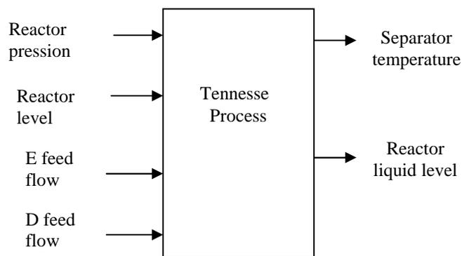
Fig. 3: Scheme input /output of Tennessee process
