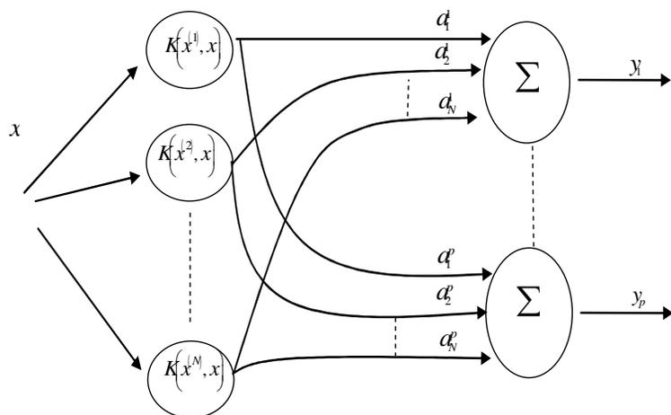
Fig1. Network of kernels functions for the MIMO modelling
