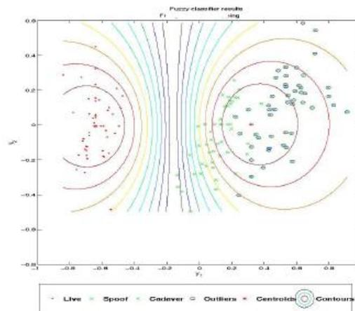
**Figure 2** Result of the FCM classifier. The left centroid is for live fingerprints and right for not live [14].
