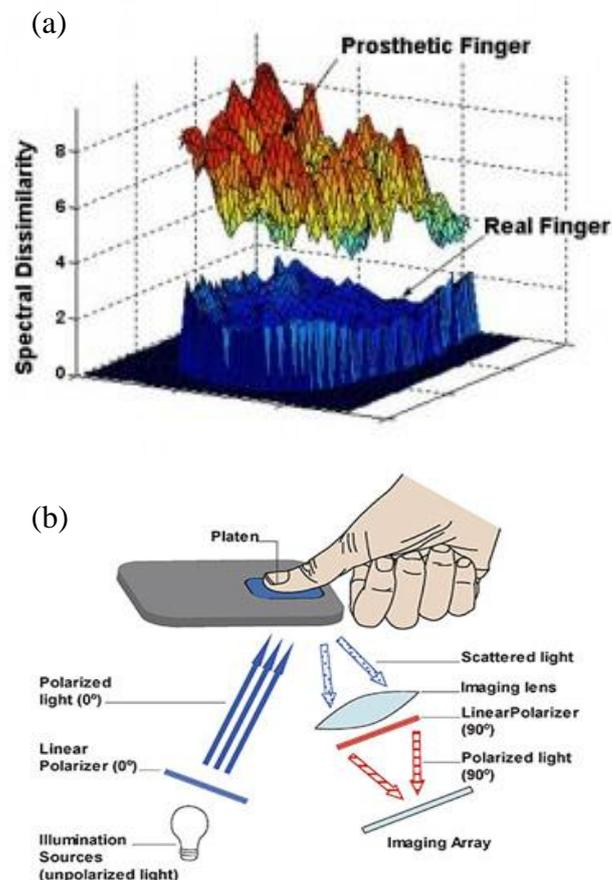
**Figure 3 a:** Spectral-characteristics-of-spoofs and real fingerprint [19] and **b:** Schematic of multispectral imaging elements [20]
