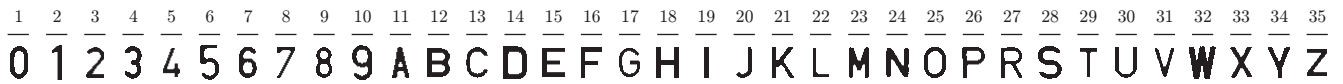
Figure 7: The template matching symbol library for the DIN-1451 Mittelschrift license plate font standard
