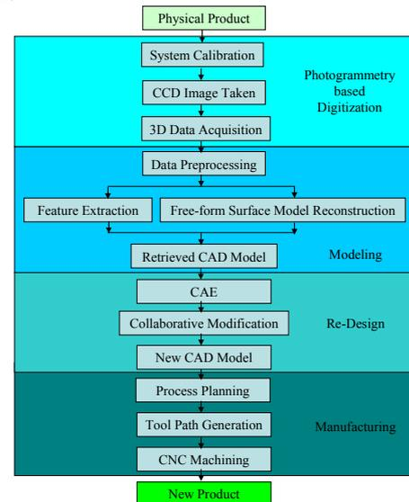
Figure 1 The overall flowchart of photogrammetry based reverse engineering system
