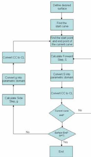
Figure 3. Overall procedure of tool path generation
