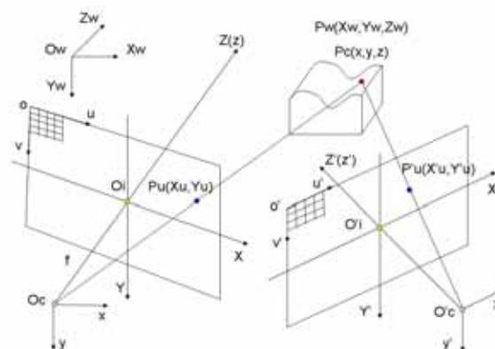
Figure 2 Pinhole camera model and geometric relationship.
